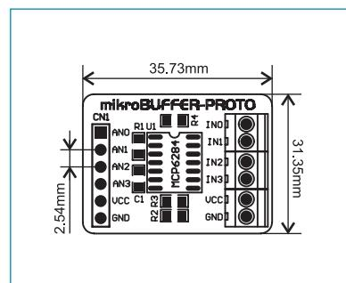
Figure 3: Dimensions of the board
