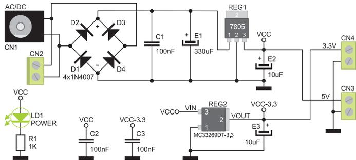
Figure 2: 5V-3.3V REG additional board connection schematic
