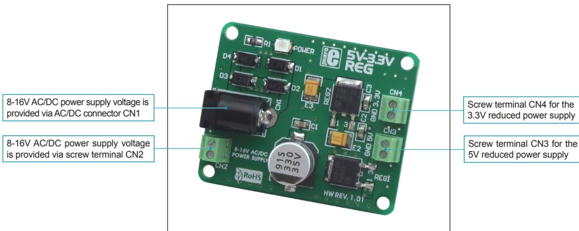
Figure 1: 5V-3.3V REG additional board
