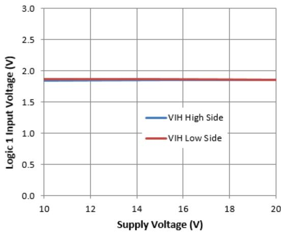
**Figure 21.** Logic 1 Input Voltage vs. Supply Voltage
