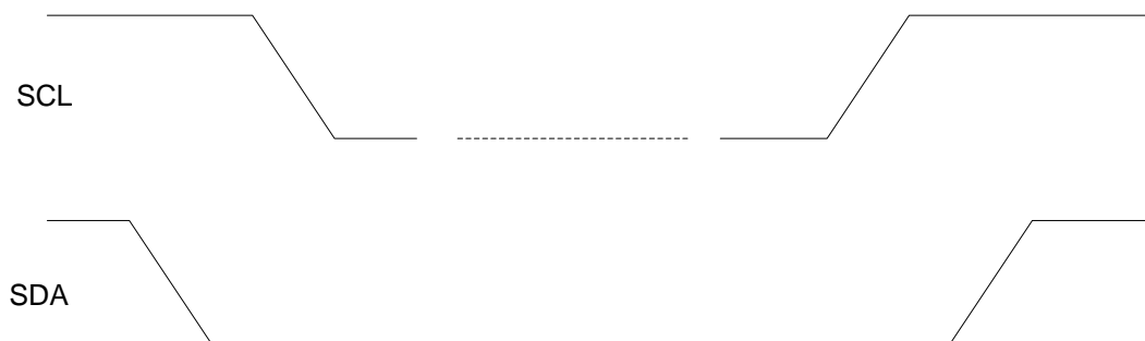
Figure 42: Timing of 2-WIRE START and STOP Condition
