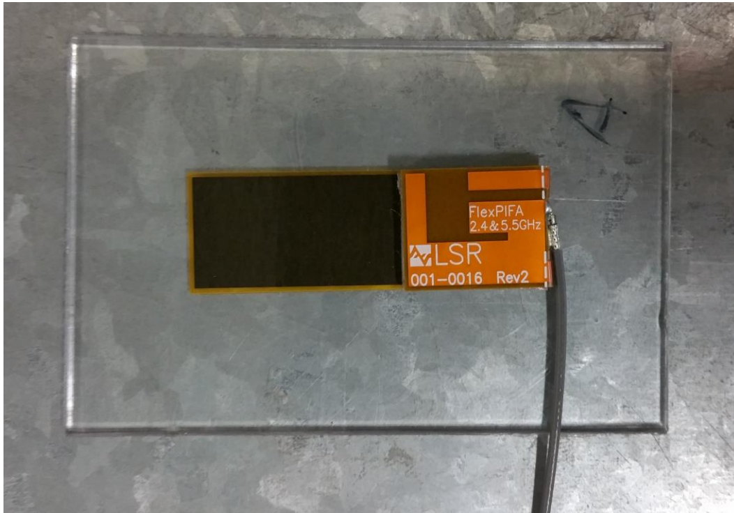
Figure 28 FlexPIFA Mounted on Metal Surface with 1.5mm Thick Polycarbonate Spacer
