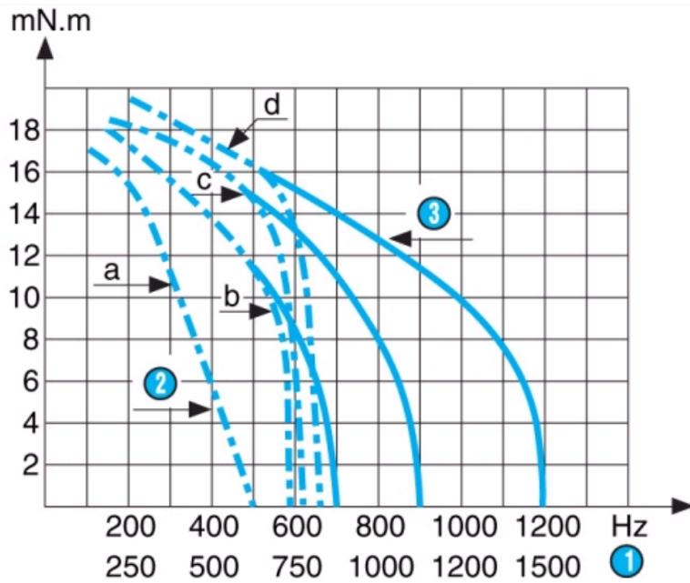
Inertia of measuring chain : 1,5 g.cm<sup>2</sup> a = constant voltage controller with R<sub>s</sub> (resistance in series) = 0 b = constant voltage controller with R<sub>s</sub> (resistance in series) = R motor c = constant voltage controller with R<sub>s</sub> (resistance in series) = 2R motor d = constant voltage controller with R<sub>s</sub> (resistance in series) = 3R motor The measurements are made with full stepping, 2-phases energised.
