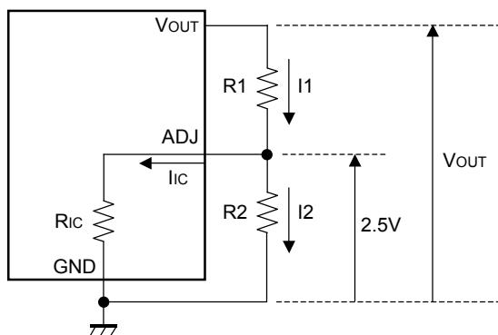
The Output Voltage of Regulator in R1154xxxxC may be adjustable for any output voltage between its 2.5V reference and its  $V_{DD}$  setting level. An external pair of resistors is required, as shown in Figure 1. The complete equation for the output voltage is described step by step as follows;
