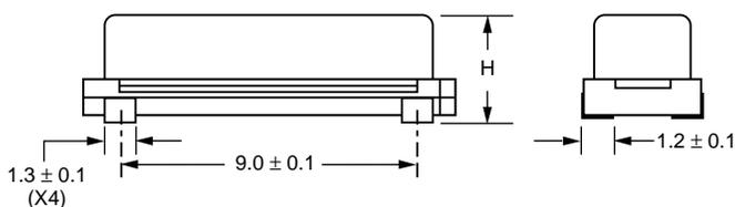
Figure 1) CSM-4A - Top, Side and End views
