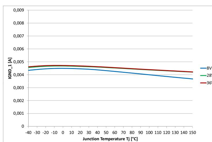
**Figure 31 Current Consumption for Whole Device with Load. One Channel Active  $I_{GND\_1} = f(T_j; V_s)$**
