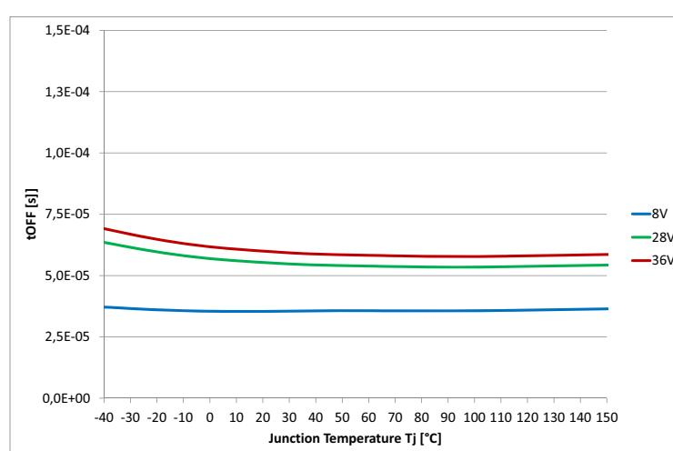
Figure 38 Turn OFF  $t_{\text{OFF}} = f(T_j; V_s)$ ,  $R_L = 12 \Omega$
