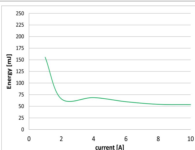
**Figure 12 Maximum Energy Dissipation Single Pulse,  $T_{J\_START} = 150^\circ\text{C}$ ;  $V_S = 28 \text{ V}$**
