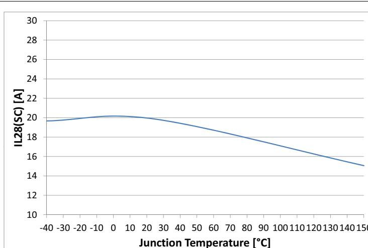
Figure 43 Overload Condition in the High Voltage Area  $I_{L28(SC)} = f(T_j; V_s)$
