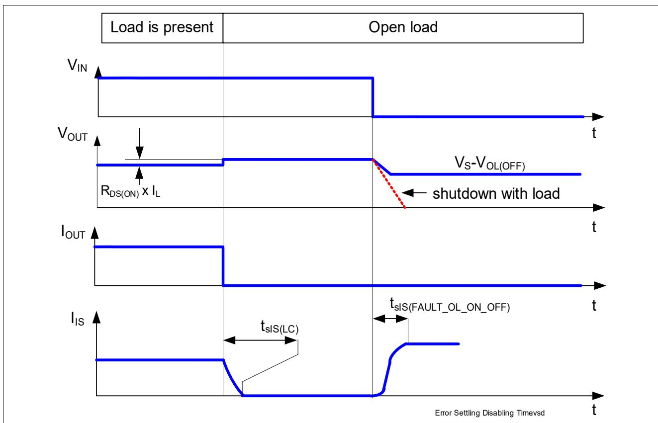
**Figure 26 SENSE Signal in Open Load Timing**
