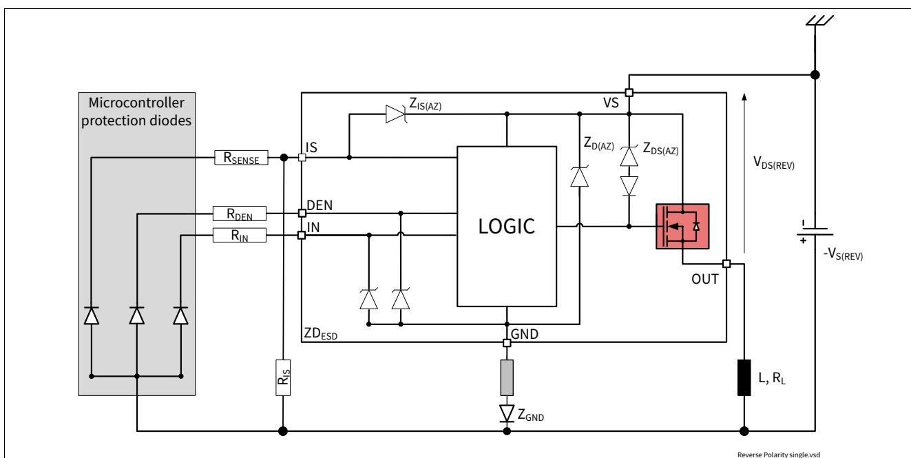
**Figure 17 Reverse Polarity Protection with External Components**
