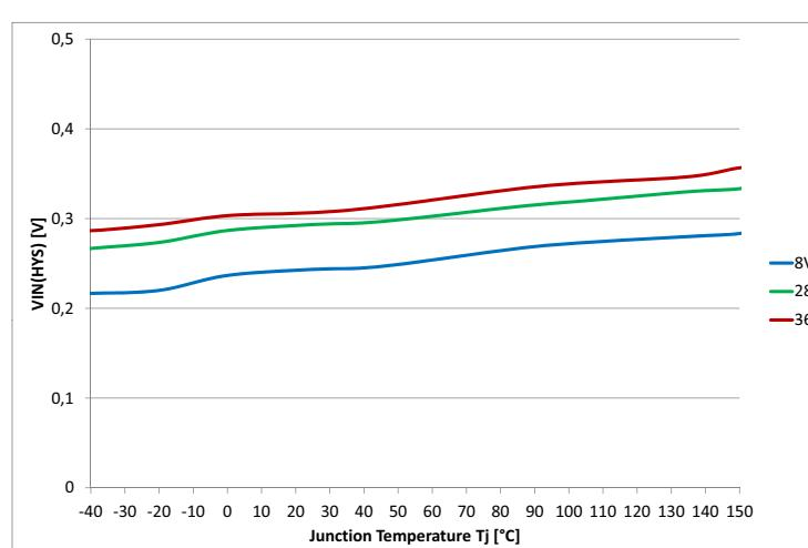
Figure 50 Input Voltage Hysteresis  $V_{IN(HYS)} = f(T_j; V_s)$
