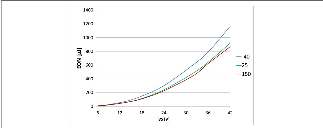
Figure 40 Switch ON Energy  $E_{ON} = f(T_J; V_S)$ ,  $R_L = 12 \Omega$
