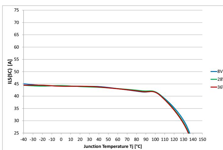
Figure 42 Overload Condition in the Low Voltage Area  $I_{L5(SC)} = f(T_j; V_s)$
