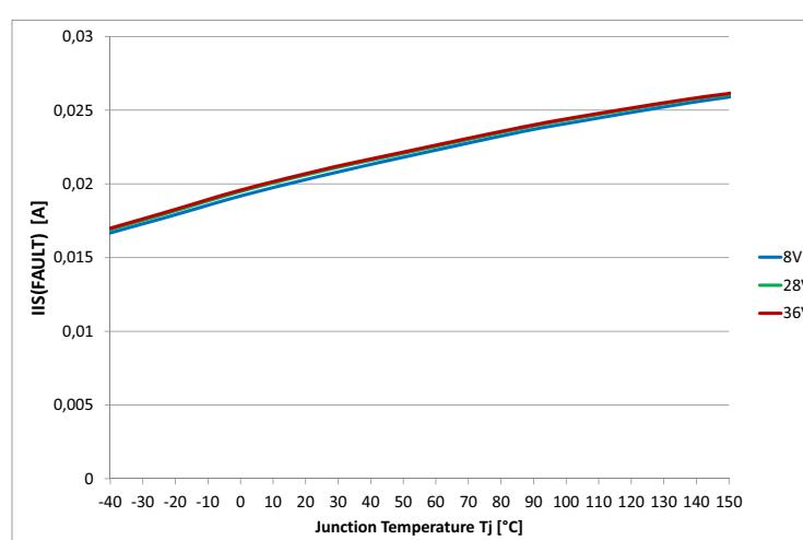
Figure 47 Sense Signal Maximum Current in Fault Condition  $I_{ISFAULT} = f(T_j; V_S)$
