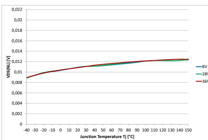
**Figure 33 Output Voltage Drop Limitation at Low Load Current  $V_{DS(NL)} = f(T_J)$  and  $V_{DS(NL)} = f(V_S)$**
