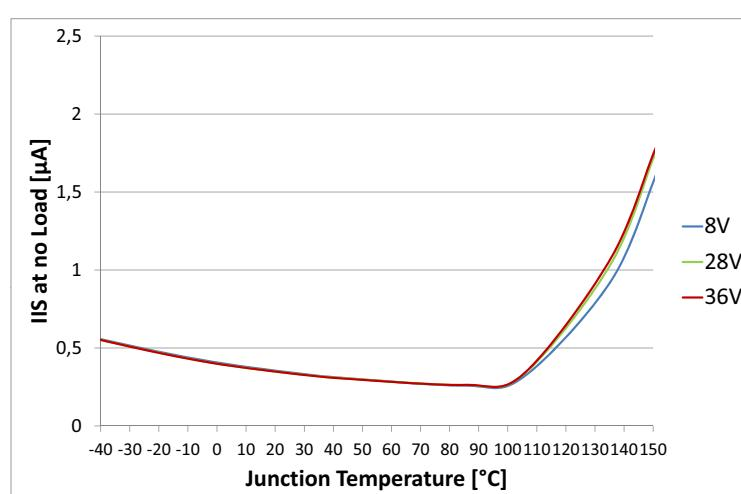
Figure 44 Current Sense at no Load  $I_{IS} = f(T_J; V_S)$ ,  $I_L = 0 \text{ A}$
