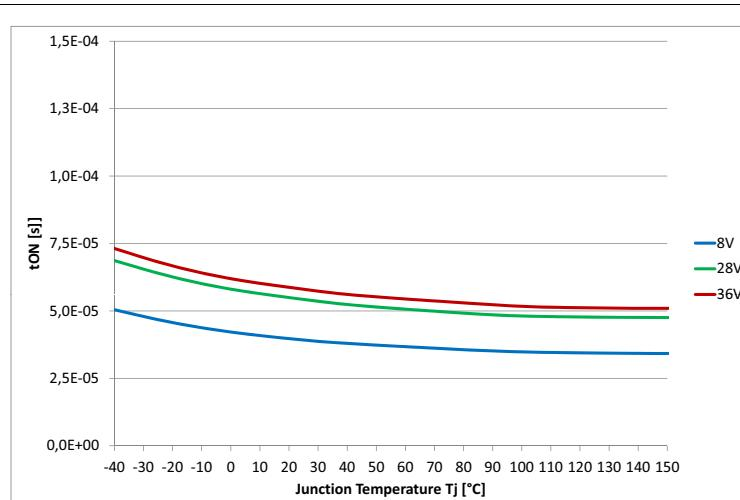
Figure 37 Turn ON  $t_{\text{ON}} = f(T_j; V_s)$ ,  $R_L = 12 \Omega$
