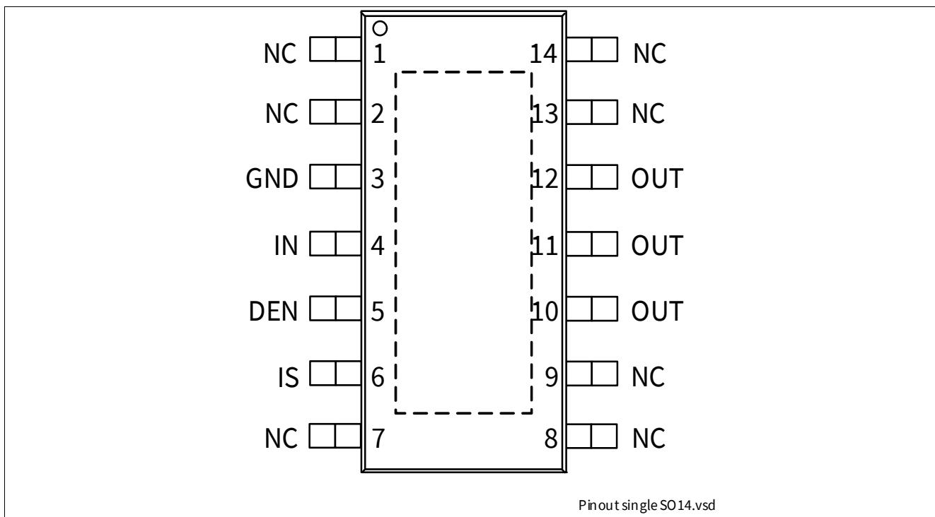
**Figure 2 Pin Configuration**
