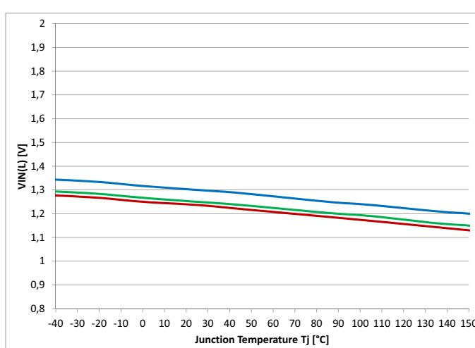
**Figure 48** Input Voltage Threshold  $V_{IN(L)} = f(T_J; V_S)$
