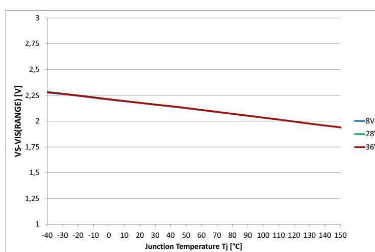
Figure 46 Sense Signal Maximum Voltage  $V_S - V_{IS(RANGE)} = f(T_j; V_S)$
