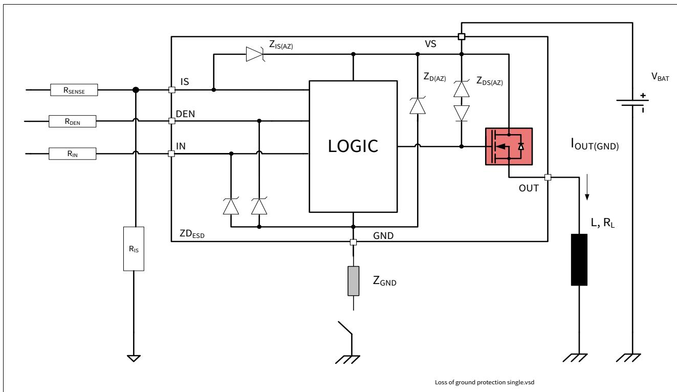
**Figure 14 Loss of Ground Protection with External Components**
