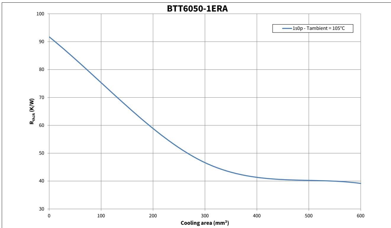
**Figure 7** Typical Thermal Resistance. PCB set-up 1s0p
