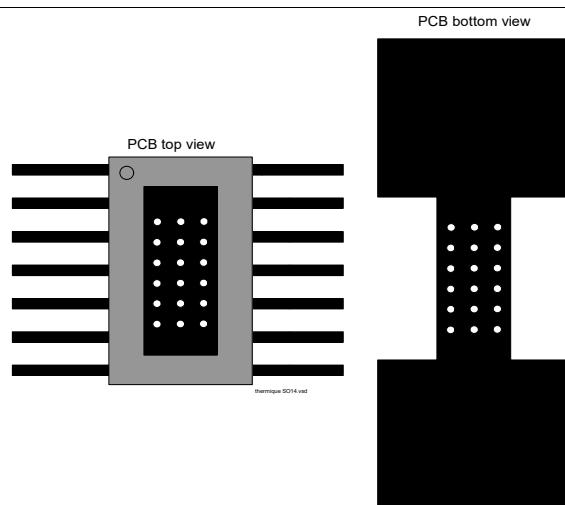
**Figure 5 PC Board Top and Bottom View for Thermal Simulation with 600 mm<sup>2</sup> Cooling Area**
