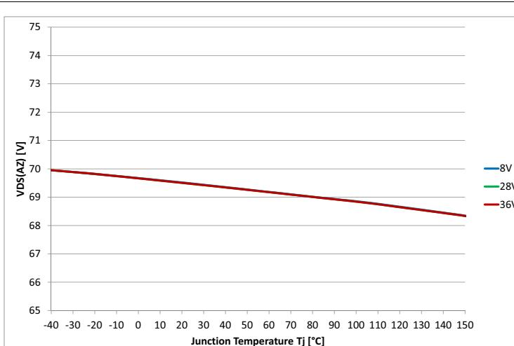
**Figure 34 Drain to Source Clamp Voltage  $V_{DS(AZ)} = f(T_J)$**
