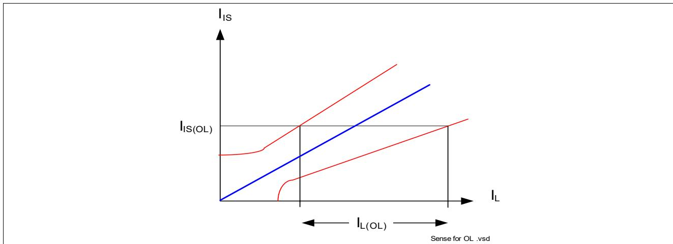
**Figure 24 Current Sense Ratio for Low Currents**
