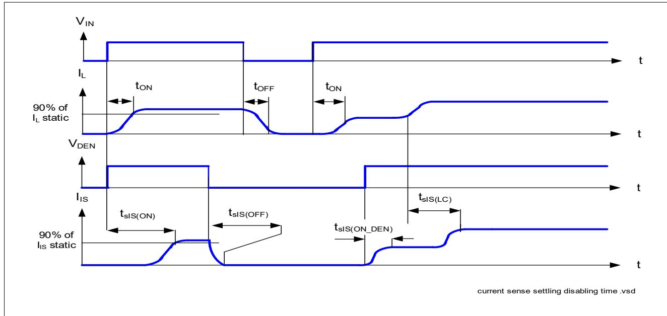
**Figure 23 Current Sense Settling / Disabling Timing**
