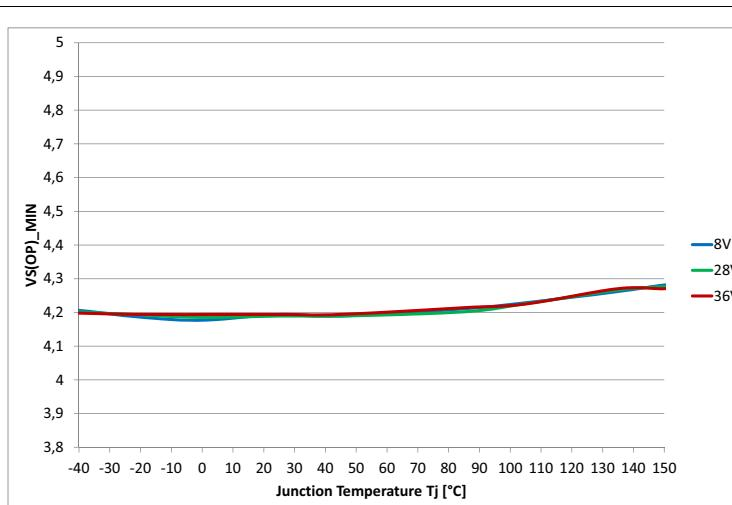
Figure 29 Minimum Functional Supply Voltage  $V_{S(OP)}_{MIN} = f(T_J)$
