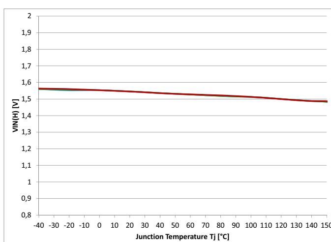
**Figure 49** Input Voltage Threshold  $V_{IN(H)} = f(T_J; V_S)$
