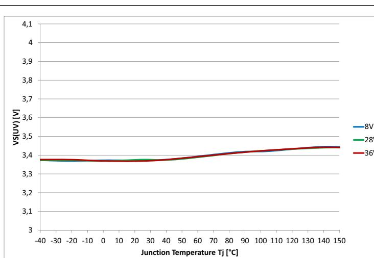
Figure 30 Undervoltage Threshold  $V_{S(uv)} = f(T_J)$
