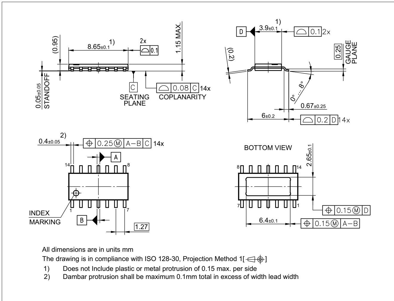
**Figure 53 PG-TDSO-14<sup>1)</sup> (Plastic Dual Small Outline Package) (RoHS-Compliant)**
