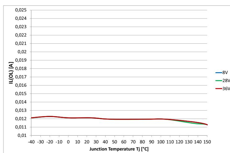
Figure 45 Open Load Detection ON State Threshold  $I_{L(OL)} = f(T_J; V_S)$
