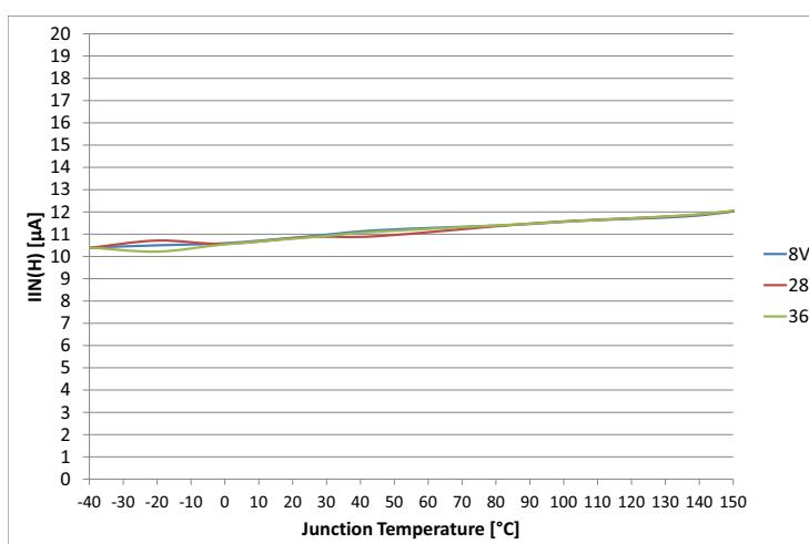
Figure 51 Input Current High Level  $I_{IN(H)} = f(T_j; V_s)$
