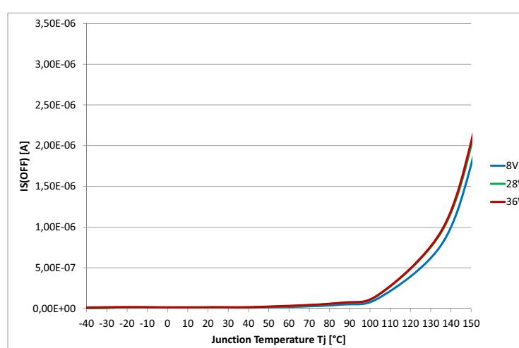
**Figure 32 Standby Current for Whole Device with Load.  $I_{S(OFF)} = f(T_j; V_s)$**
