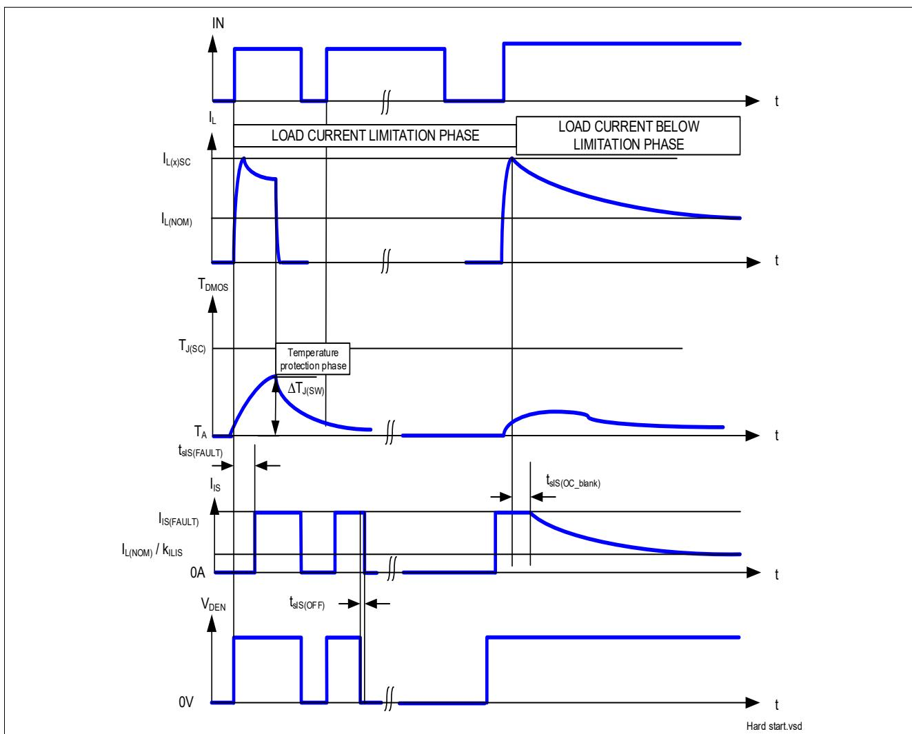
**Figure 19 Overload Protection**
