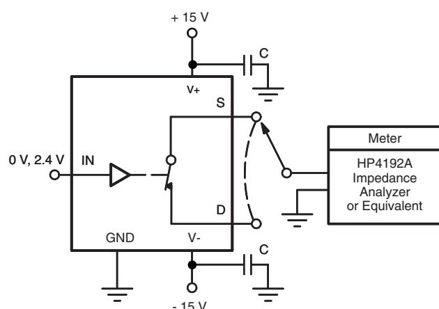
Figure 5. Source/Drain Capacitances
