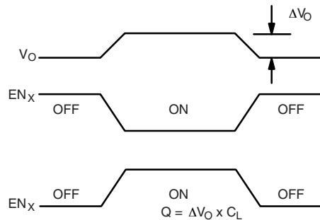
Figure 3. Charge Injection
