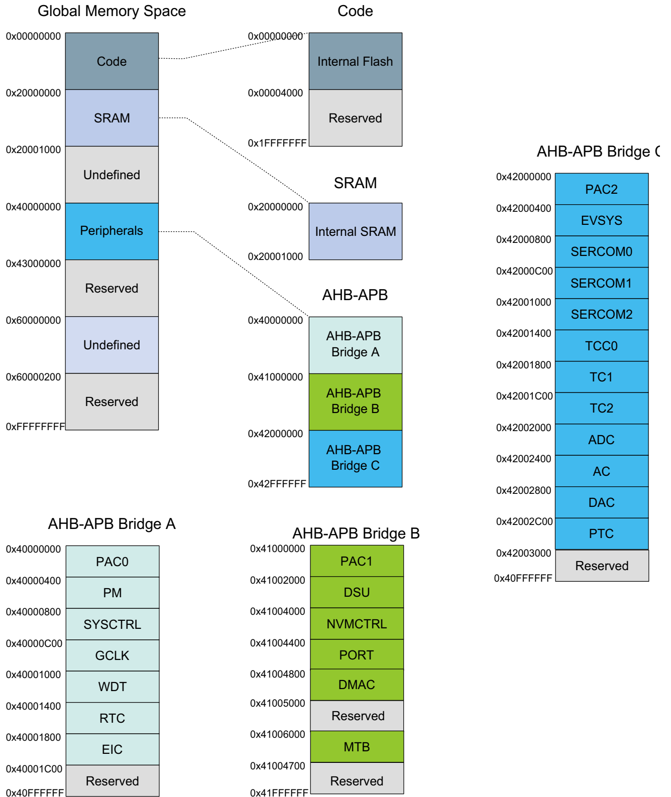
Figure 8-1. Atmel SAM D10 Product Mapping
