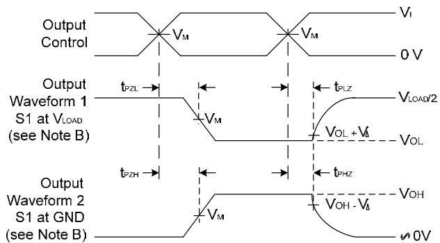
Figure 1. Load Circuit and Voltage Waveforms
