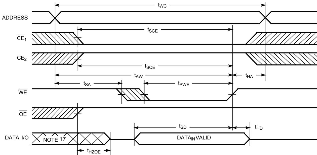
**Write Cycle No.3 ( $\overline{WE}$  Controlled,  $\overline{OE}$  LOW)<sup>[15, 16]</sup>**
