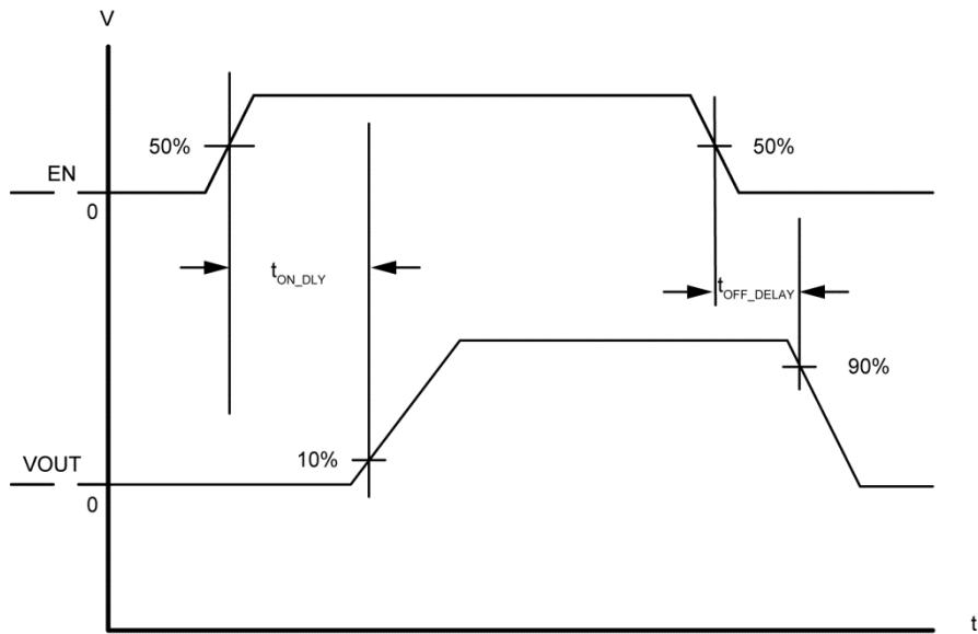
Figure 2. Turn-On/Off Delay
