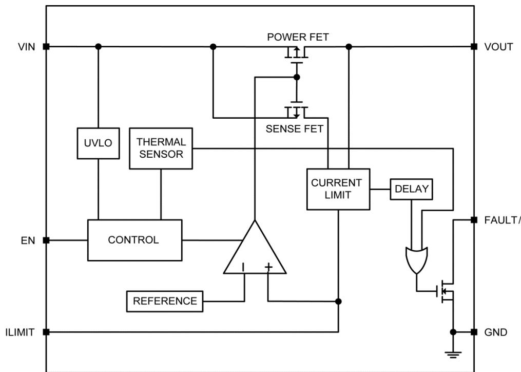
Figure 5. MIC2039 Block Diagram
