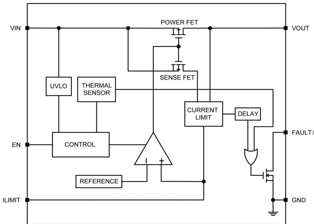
Figure 5. MIC2039 Block Diagram
