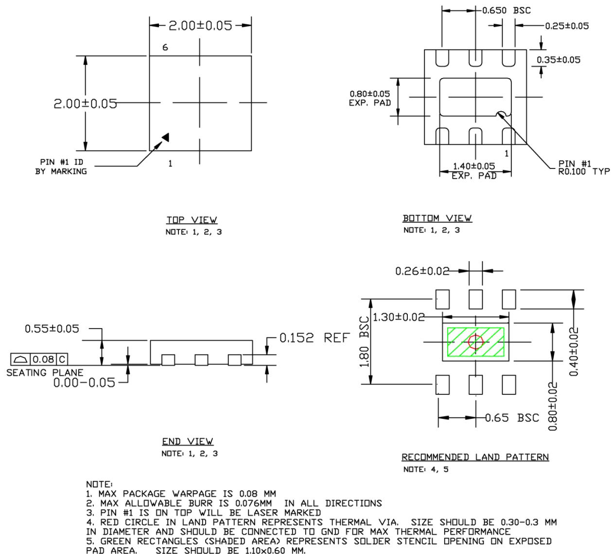
6-Pin 2mm x 2mm Thin DFN (MT)
