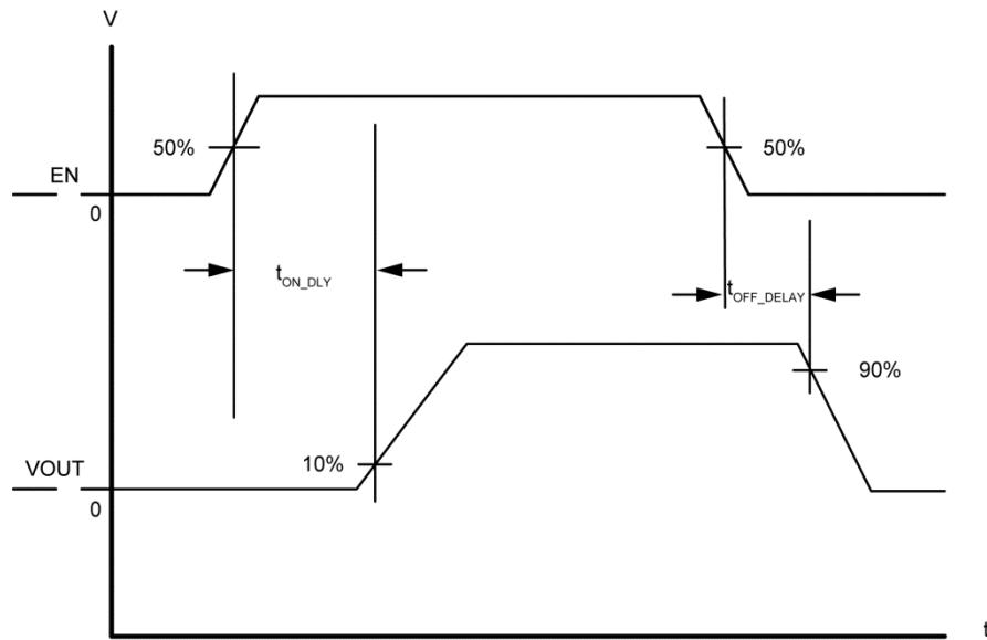
Figure 2. Turn-On/Off Delay
