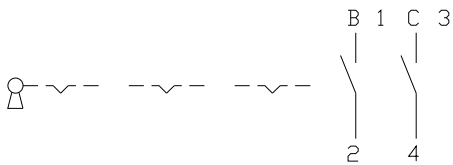
20 Keylock switch 2 positions page 39
