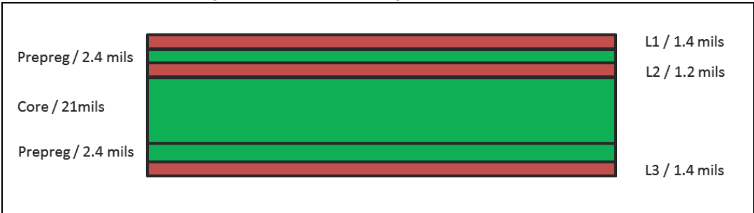
Figure 18. PCB stack-up recommendation
