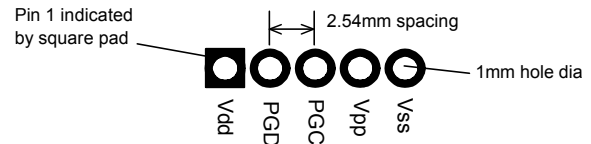
Figure 13. Recommended plate-through connector design
