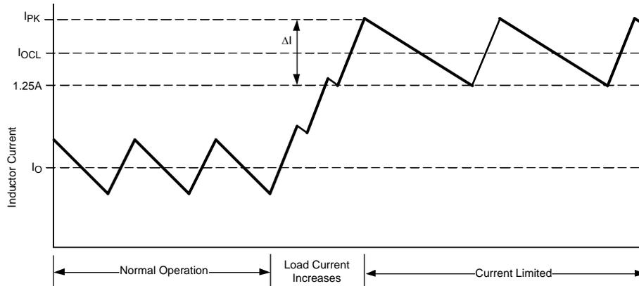
**Figure 7. Inductor Current - Current Limit Operation**
