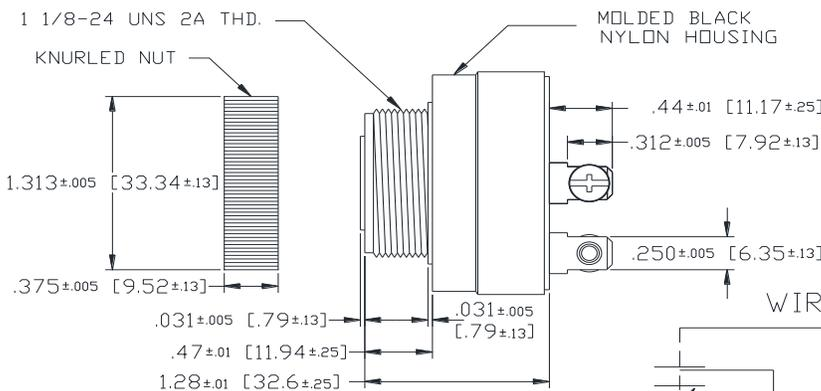
NOTE B: MOUNTING- REMOVE BLACK PLASTIC NUT AND INSERT THREADED FRONT THROUGH 1.25" HOLE PUNCHED IN PANEL, IF ORIENTATION IS NEEDED, NOTE LOCKING FLATS ON DRAWING. SCREW NUT BACK ON. DO NOT OVERTIGHTEN.
