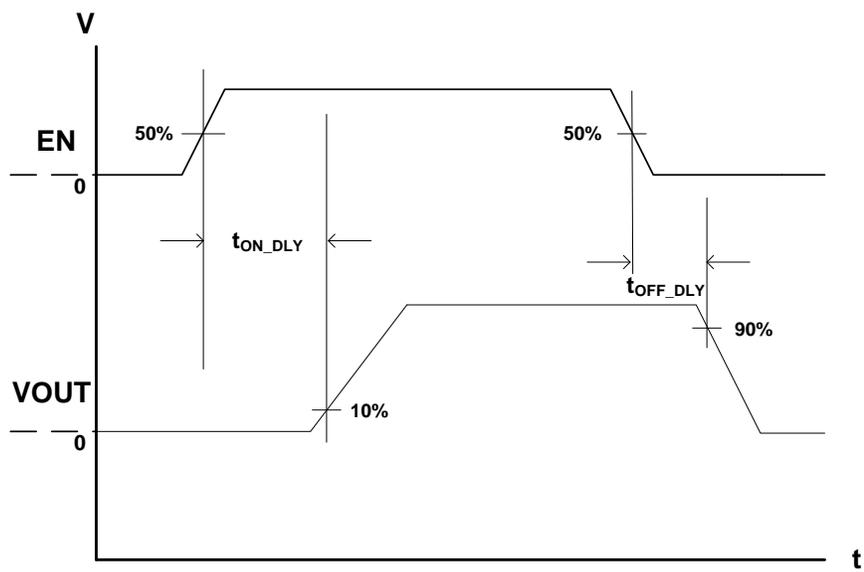
Figure 2. Turn-On/Off Delay
