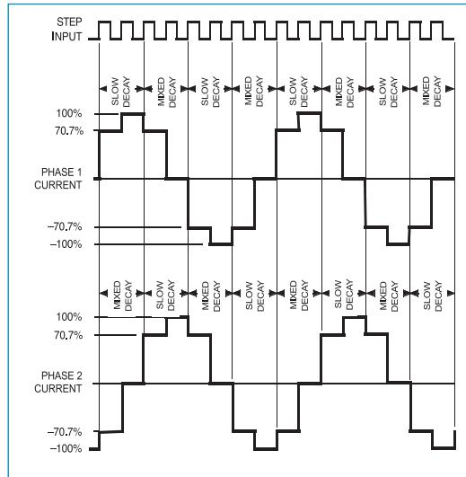
Figure 5: Half Step mode: MS1=1, MS2=0, DIR=1
