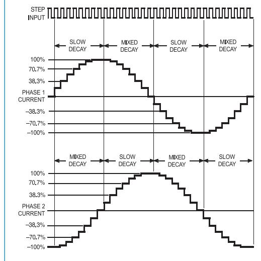
Figure 7: 8 Microstep mode: MS1=1, MS2=1, DIR=1
