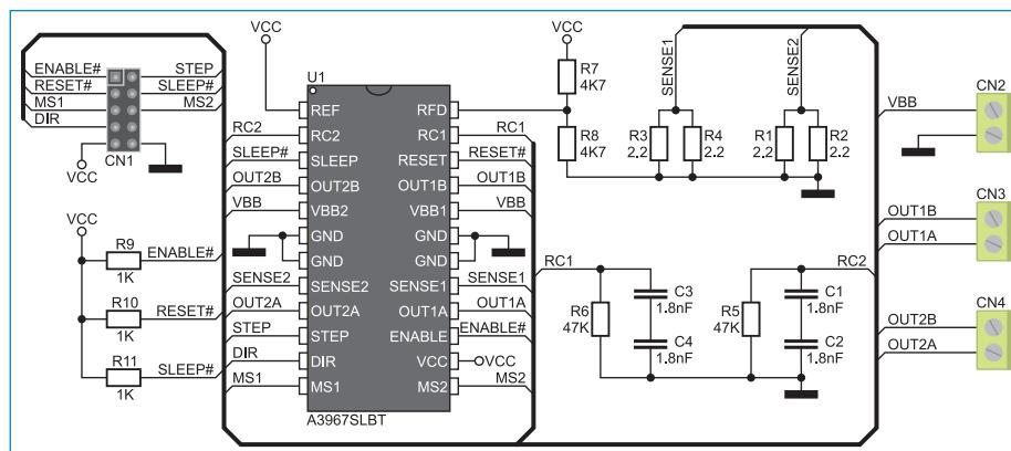
Figure 3: Bipolar Stepper Motor Driver connection schematic
