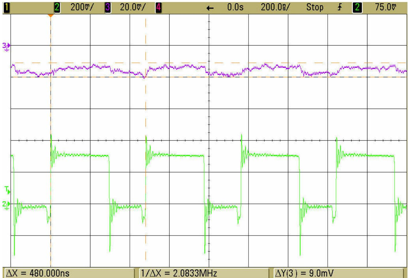
Figure 3. Switch Node &amp; Output Ripple Voltage Waveforms
