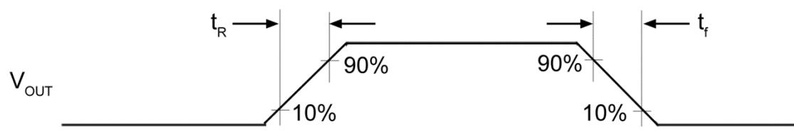
Figure 1. Output Voltage Rise and Fall time Measurements
