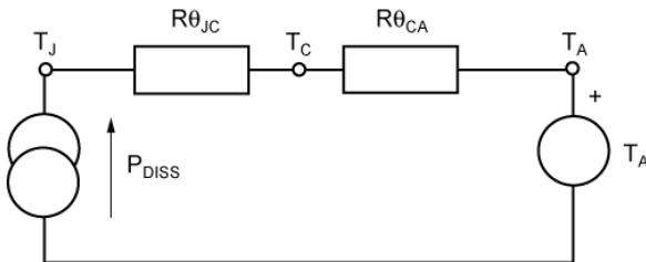
**Figure 5. Simple Thermal Circuit**
