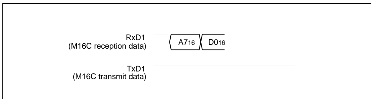
Figure 1.29.28. Timing for erasing all unlocked blocks
