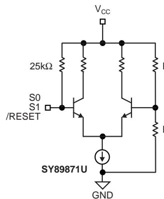
Figure 2b. Simplified TTL/CMOS Input Buffer
