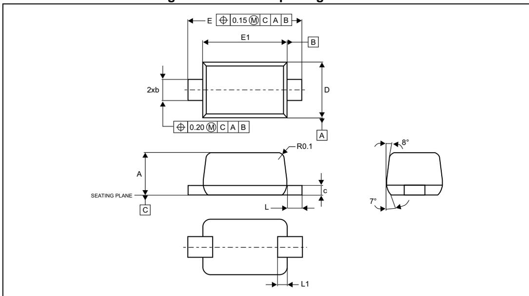
**Table 6. SOD-523 package mechanical data**
