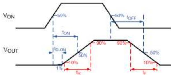
Test conditions:  $T_A = +25^\circ\text{C}$ ,  $C_{IN} = 1\mu\text{F}$ ,  $C_L = 0.1\mu\text{F}$ ,  $R_L = 10\Omega$  (unless otherwise specified).
