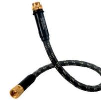
The only VNA microwave cable worldwide with a typical 50 ppm phase variation vs. temperature between +15 and +30 °C only. No "PTFE phase knee" at +19 °C as on conventional VNA test cable assemblies which cause phase variations and unstable measurements in critical laboratory conditions.
