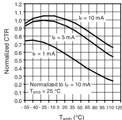
Normalized CTR vs. Ambient Temperature
