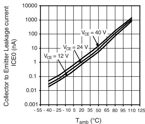
Figure 5. Collector to Emitter Leakage Current vs.
