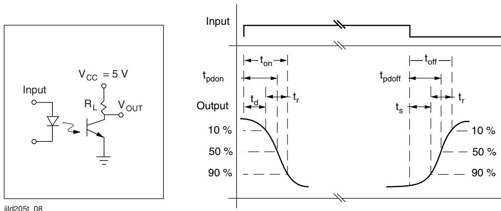
Figure 2. Switching Test Circuit
