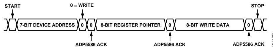
Figure 24. I 2 C Single Byte Write Sequence
