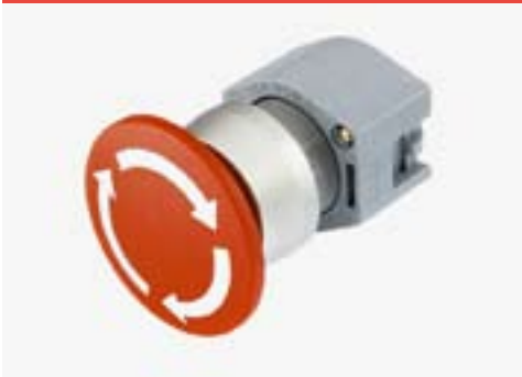
Stop switch, twist release, mushroom head, 40 mm diameter, 22.5 mm mounting
