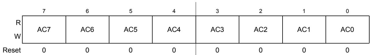
**Figure 11-21. MSCAN Identifier Acceptance Registers (Second Bank) — CANIDAR4–CANIDAR7**
