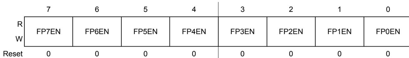
Figure 14-5. LCD Frontplane Enable Register 0 (LCDFPENR0)
