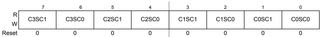
**Figure 6-9. Debug State Control Register 1 (DBGSCR1)**
