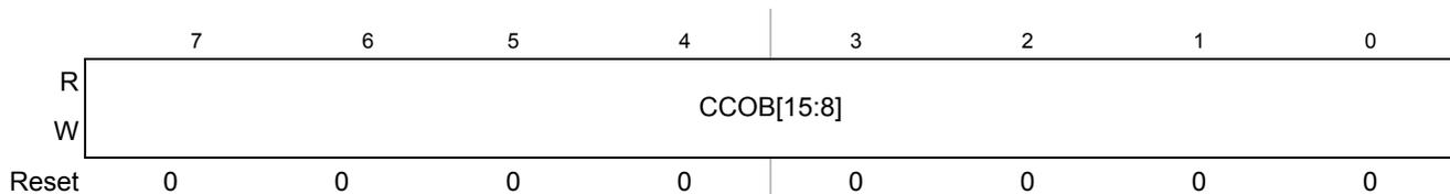
**Figure 21-22. Flash Common Command Object 2 High Register (FCCOB2HI)**
