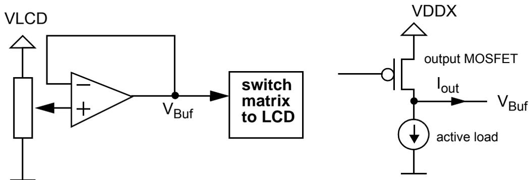
Figure E-1. Buffer configuration (left) and buffer output stage (right)
