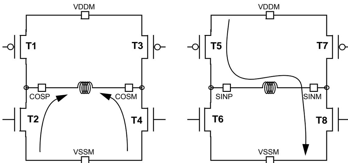
Figure 17-12. Current Flow when STEP = 1, DCOIL = 1, ITG = 0, RCIR = 1
