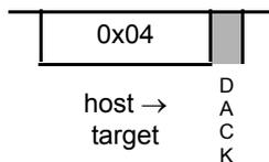
Provided ENBDC is set, the BACKGROUND command causes the target MCU to enter active BDM as soon as the current CPU instruction finishes. If ENBDC is cleared, the BACKGROUND command is ignored.
