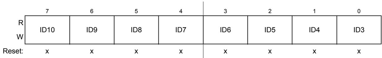
**Figure 11-30. Identifier Register 0 — Standard Mapping**
