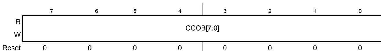
**Figure 21-19. Flash Common Command Object 0 Low Register (FCCOB0LO)**
