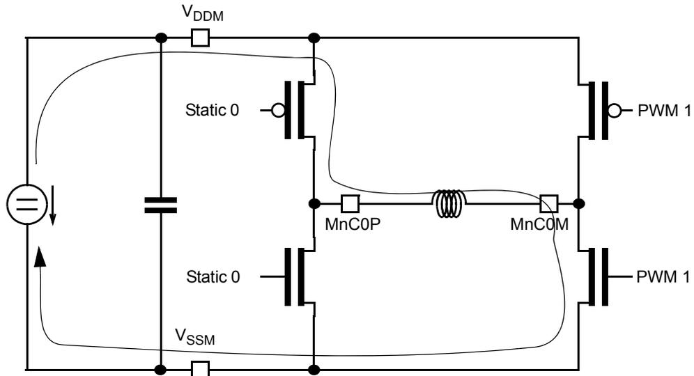
Figure 16-12. PWM Active Phase, RECIRC = 0, S = 0
