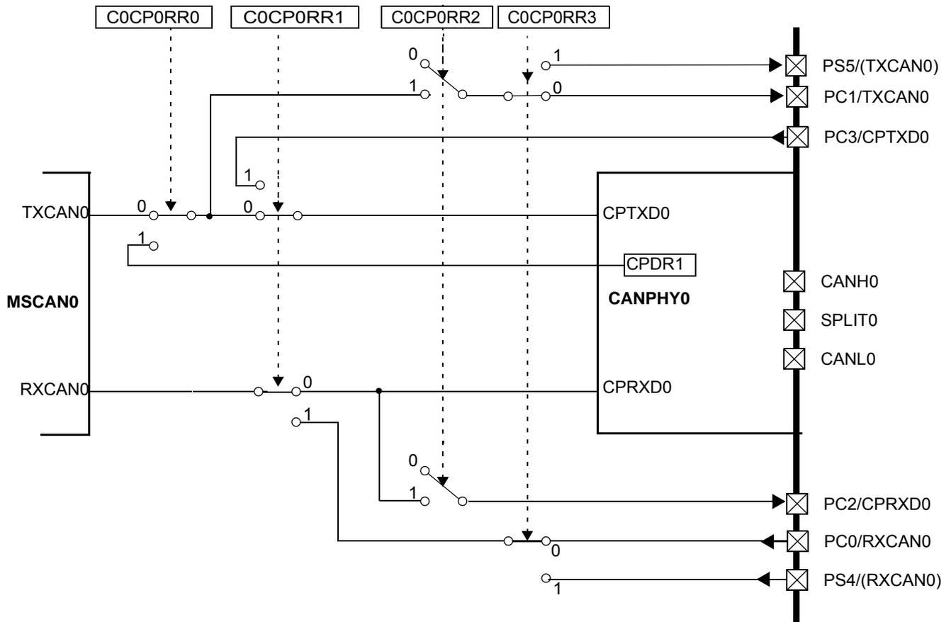
Figure 2-2. MSCAN0-CANPHY0 Routing Options Illustration
