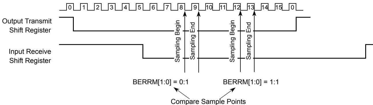
**Figure 15-19. Timing Diagram Bit Error Detection**
