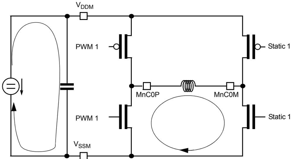
Figure 16-15. PWM Passive Phase, RECIRC = 1, S = 0
