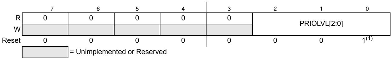
**Figure 4-12. Interrupt Request Configuration Data Register 7 (INT\_CFDATA7)**
