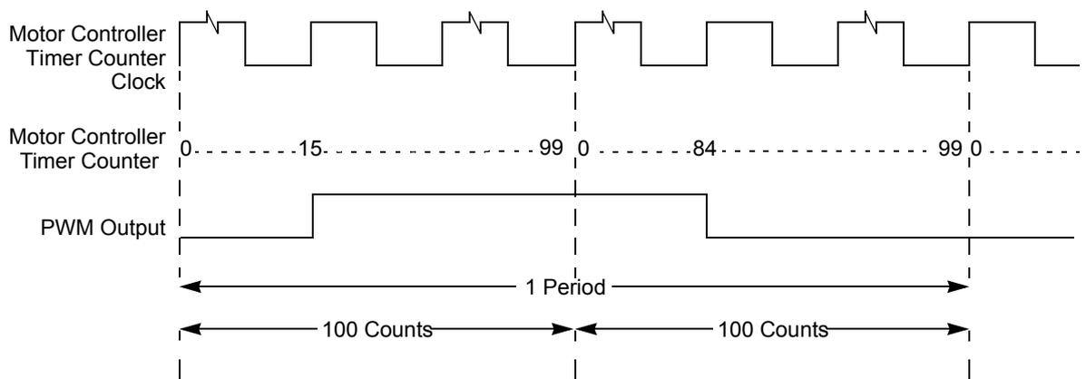
**Figure 16-21. PWM Output: DITH = 1, MCAM[1:0] = 11, MCDC = 31, MCPER = 200, RECIRC = 0**
