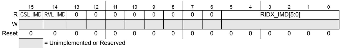
**Figure 10-16. ADC Intermediate Result Information Register (ADCIMDRI)**
