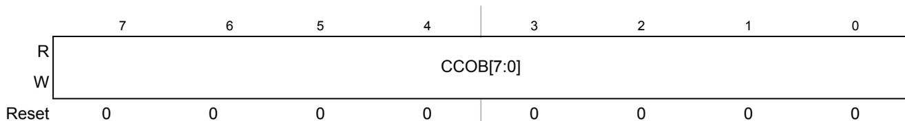
**Figure 21-25. Flash Common Command Object 3 Low Register (FCCOB3LO)**
