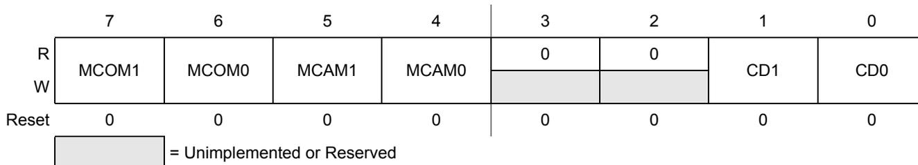
Figure 16-7. Motor Controller Control Register Channel 0–7 (MCCC0–MCCC7)
