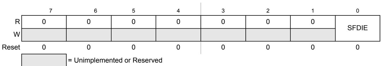
**Figure 21-10. Flash Error Configuration Register (FERCNFG)**
