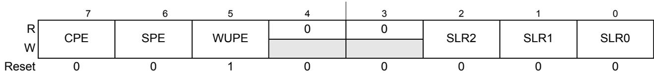
**Figure 22-3. CAN Physical Layer Control Register (CPCR)**
