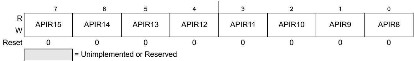
Figure 7-23. Autonomous Periodical Interrupt Rate High Register (CPMUAPIRH)
