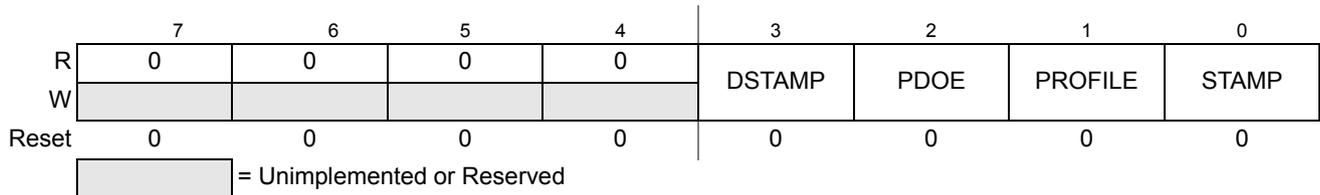
**Figure 6-6. Debug Trace Control Register Low (DBGTCRL)**
