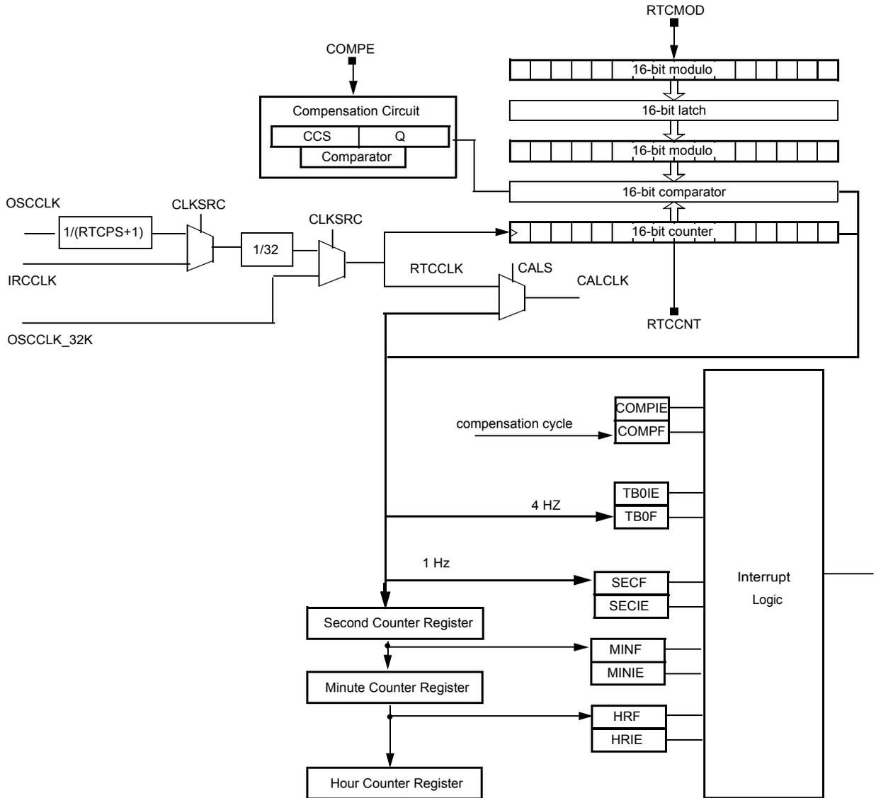
Figure 18-1. Real-Time Counter with Calendar (RTC) Block Diagram
