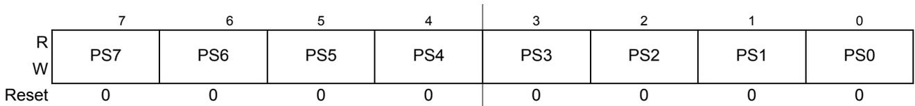
Figure 19-6. SSG Clock Prescaler Register (SSGPSL)
