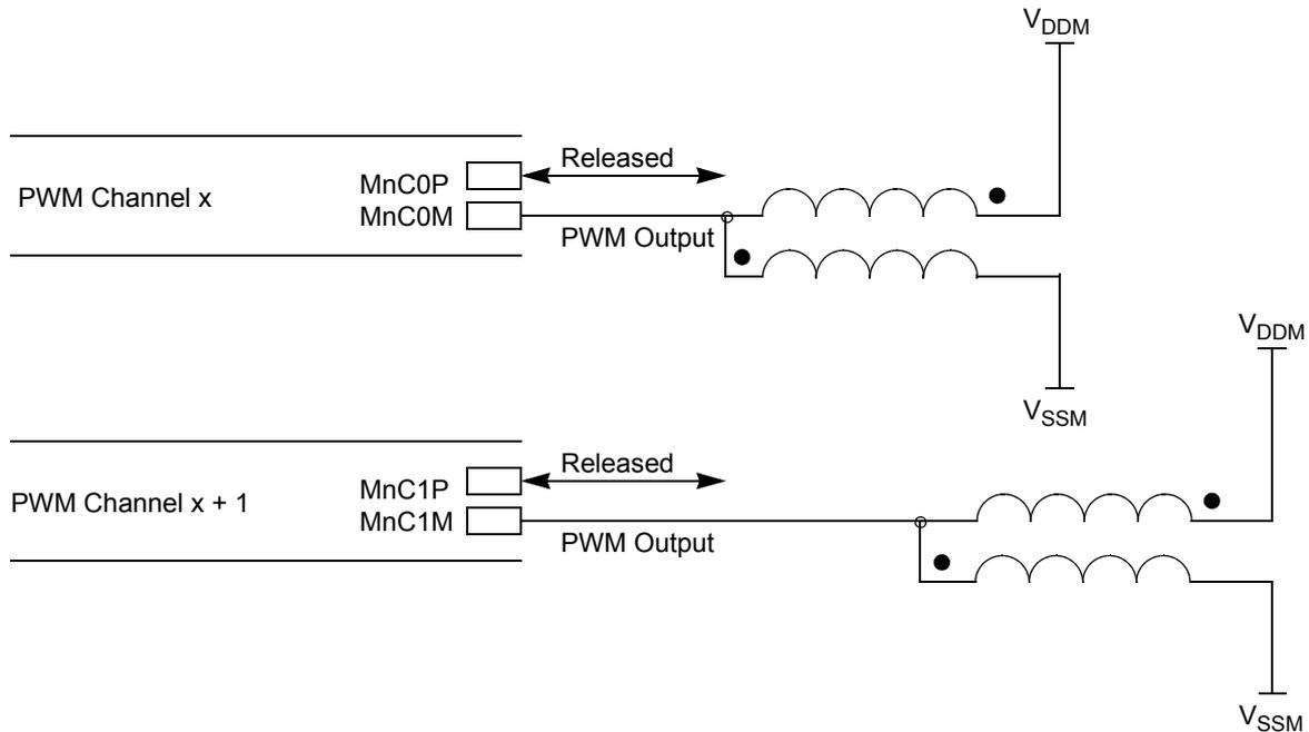
Figure 16-11. Typical Quad Half H-Bridge Mode Configuration
