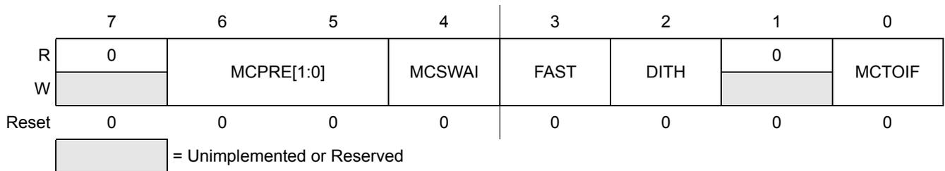
Figure 16-3. Motor Controller Control Register 0 (MCCTL0)
