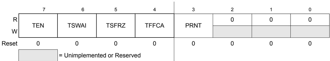
**Figure 8-12. Timer System Control Register 1 (TSCR1)**
