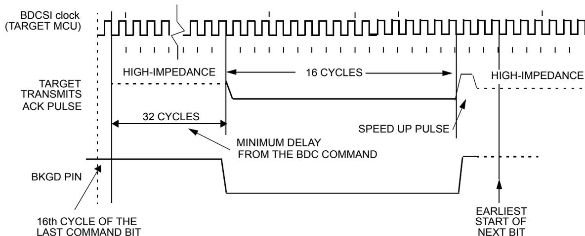
Figure 5-9. Target Acknowledge Pulse (ACK)
