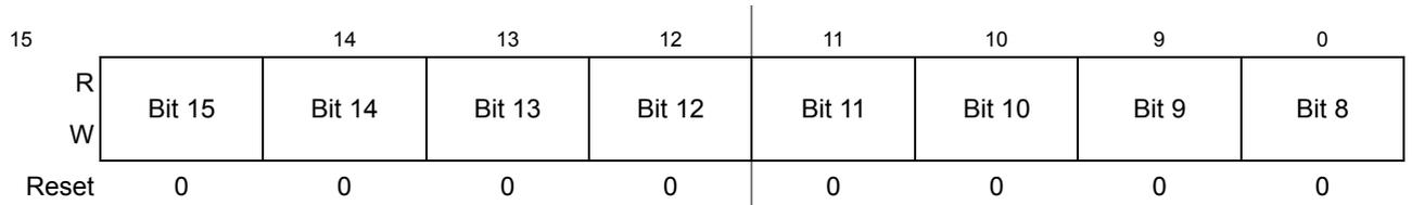
**Figure 8-22. Timer Input Capture/Output Compare Register x High (TCxH)**
