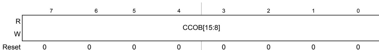
**Figure 21-18. Flash Common Command Object 0 High Register (FCCOB0HI)**
