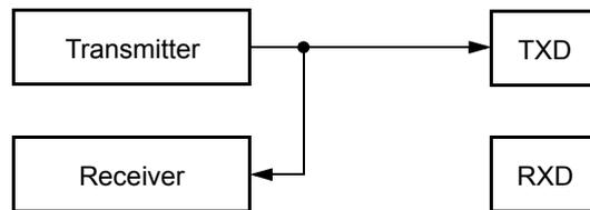
**Figure 15-31. Loop Operation (LOOPS = 1, RSRC = 0)**
