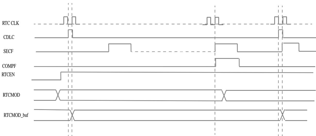
Figure 18-13. Buffered register load sequence and CDLC
