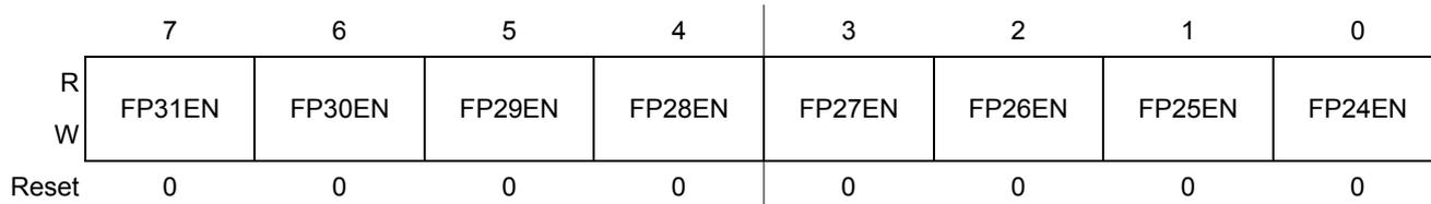
Figure 14-8. LCD Frontplane Enable Register 3 (LCDFPENR3)
