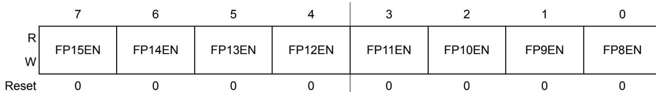
Figure 14-6. LCD Frontplane Enable Register 1 (LCDFPENR1)
