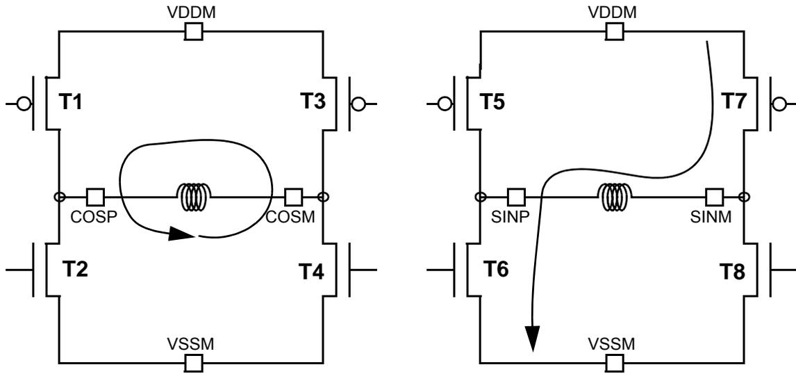
Figure 17-14. Current flow when STEP = 3, DCOIL = 1, ITG = 1
