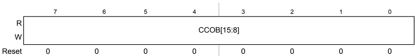
**Figure 21-28. Flash Common Command Object 5 High Register (FCCOB5HI)**
