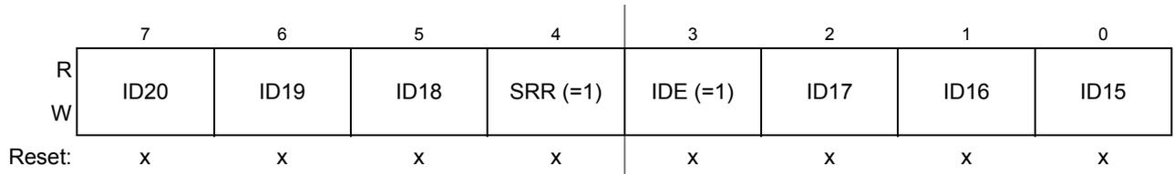
Figure 11-27. Identifier Register 1 (IDR1) — Extended Identifier Mapping
