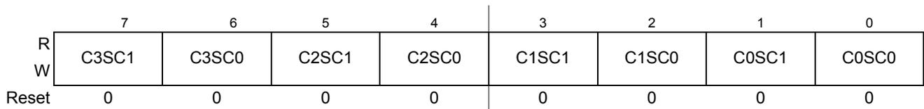
**Figure 6-11. Debug State Control Register 3 (DBGSCR3)**
