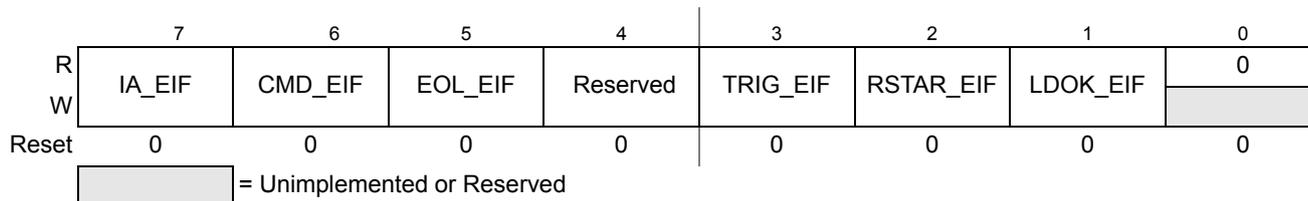
Figure 10-12. ADC Error Interrupt Flag Register (ADCEIF)
