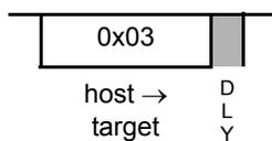
Disables the serial communication handshake protocol. The subsequent commands, issued after the ACK\_DISABLE command, do not execute the hardware handshake protocol. This command is not followed by an ACK pulse.
