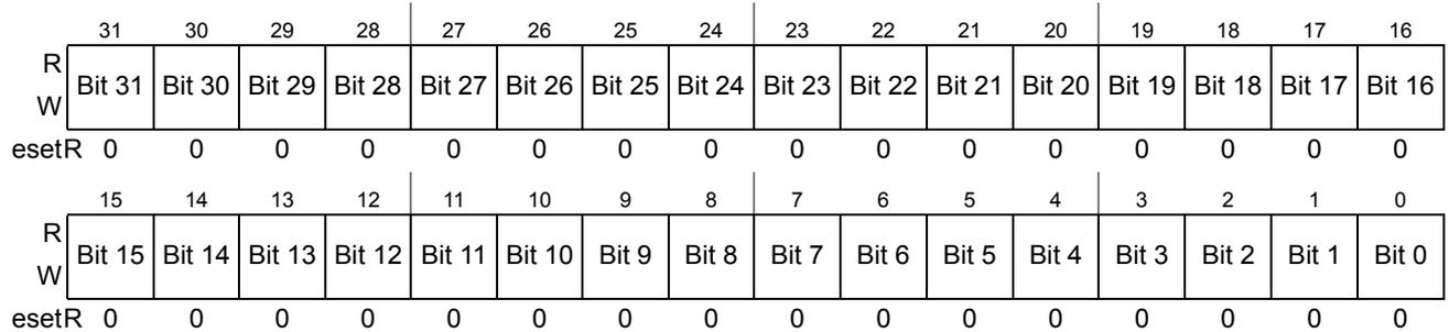
Figure 6-22. Debug Comparator C Data Register (DBGCD)
