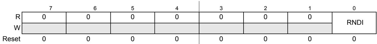
**Figure 19-17. SSG Interrupt Flag Register (SSGIF)**
