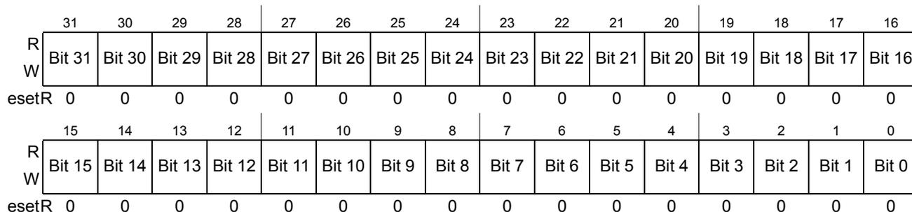
Figure 6-16. Debug Comparator A Data Register (DBGAD)
