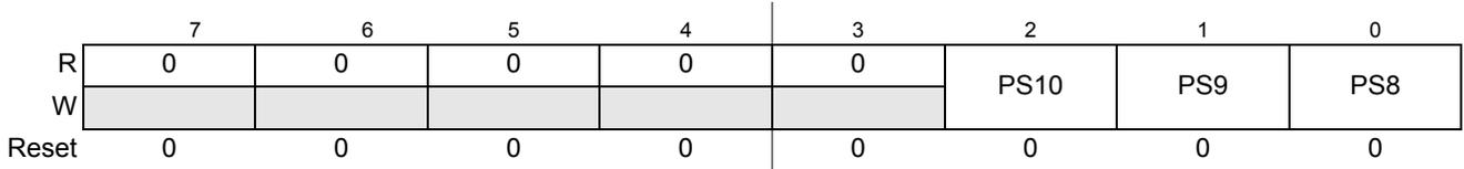
Figure 19-5. SSG Clock Prescaler Register (SSGPSH)
