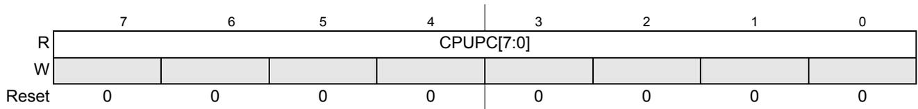
**Figure 3-7. Captured S12ZCPU Program Counter (MMCPCH, MMPCM, MMCPCL)**
