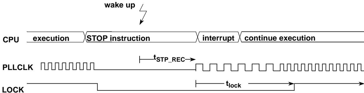
Depending on the COP configuration there might be an additional significant latency time until COP is active again after exit from Stop Mode due to clock domain crossing synchronization. This latency time occurs if COP clock source is ACLK and the CSAD bit is set (please refer to CSAD bit description for details).
