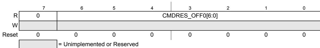
Figure 10-26. ADC Command and Result Offset Register 0 (ADCCROFF0)
