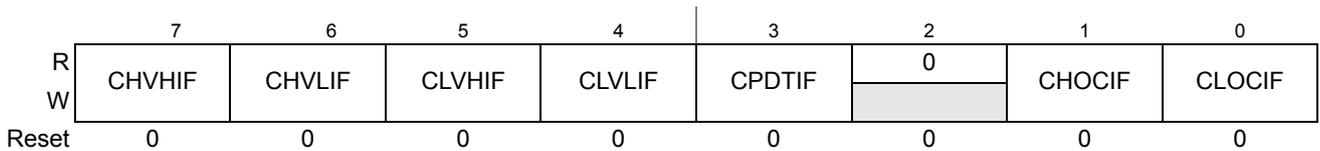
**Figure 22-9. CAN Physical Layer Interrupt Flag Register (CPIF)**
