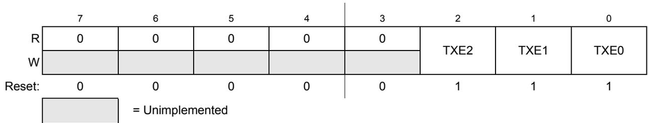
**Figure 11-10. MSCAN Transmitter Flag Register (CANTFLG)**
