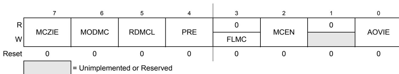
Figure 17-3. Modulus Down Counter Control Register (MDCCTL)
