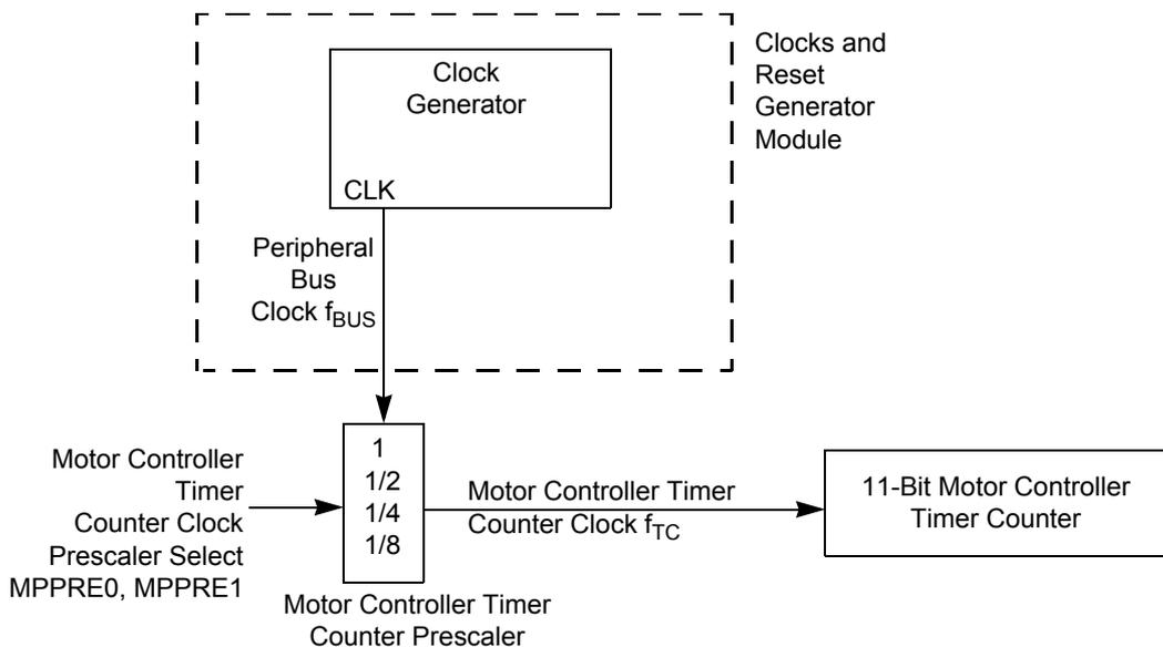
**Figure 16-22. Motor Controller Counter Clock Selection**
