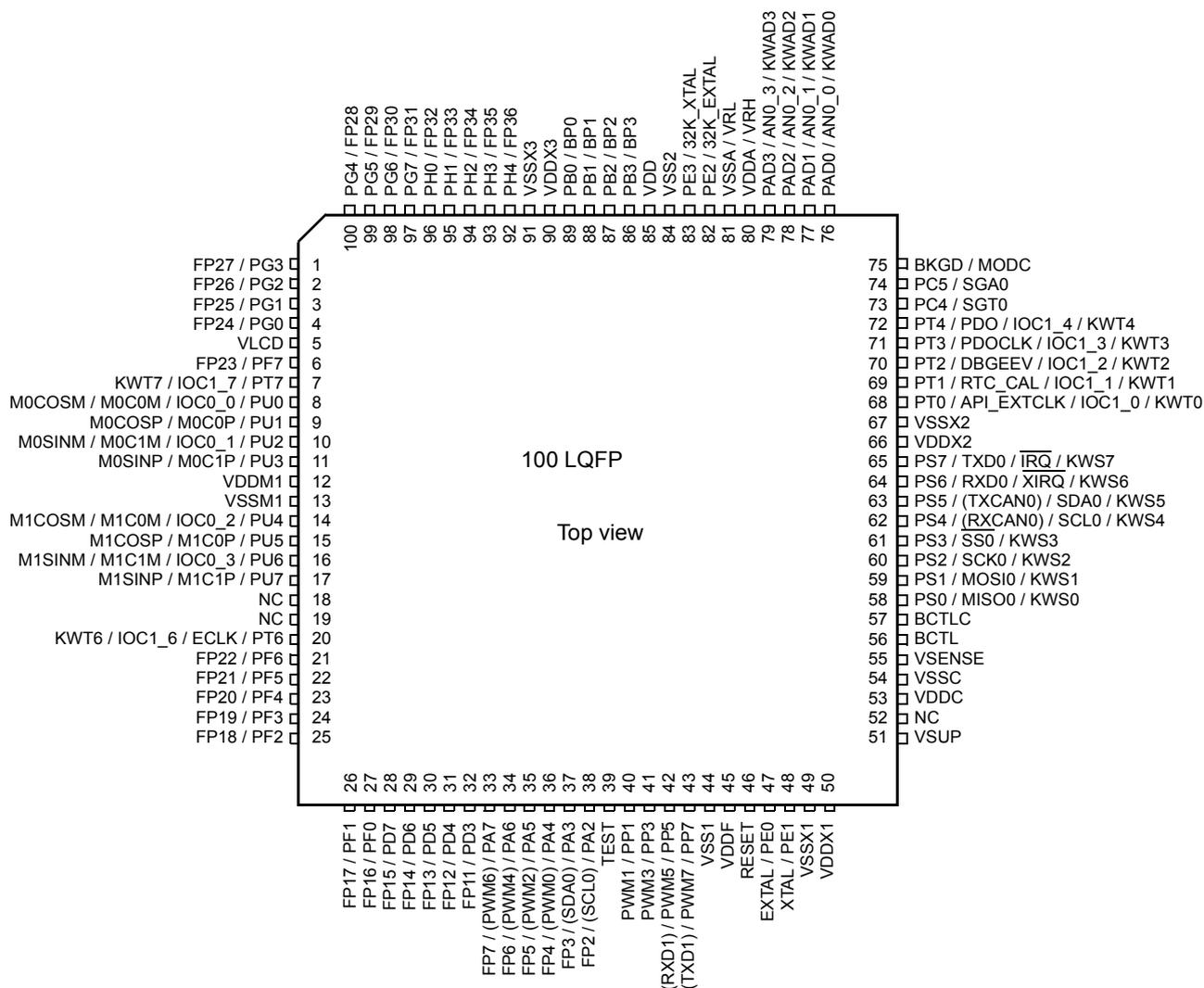
Figure 1-5. MC9S12ZVH-Family 100-pin LQFP pin out <sup>1</sup>
