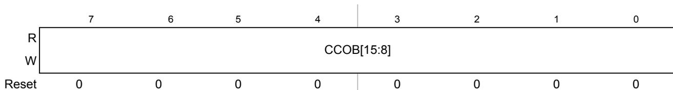
**Figure 21-26. Flash Common Command Object 4 High Register (FCCOB4HI)**
