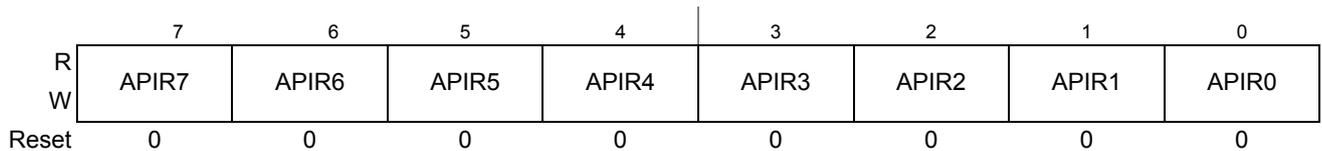
Figure 7-24. Autonomous Periodical Interrupt Rate Low Register (CPMUAPIRL)
