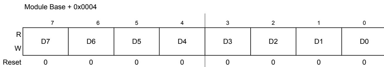
**Figure 13-8. IIC Bus Data I/O Register (IBDR)**
