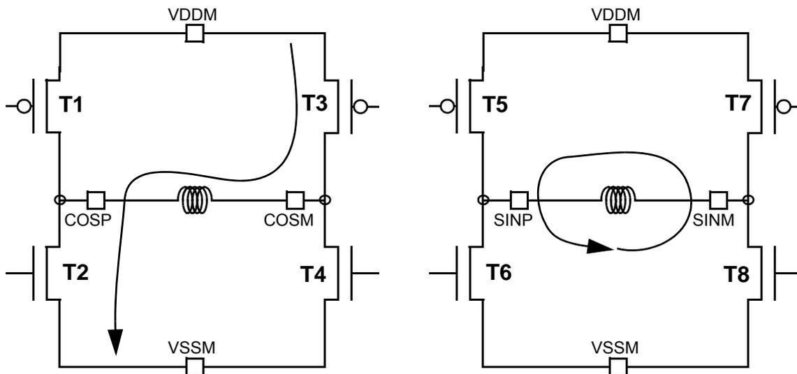
Figure 17-13. Current flow when STEP = 2, DCOIL = 1, ITG = 1
