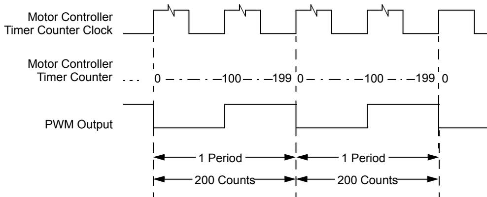
**Figure 16-17. PWM Output: DITH = 0, MCAM[1:0] = 01, MCDC = 100, MCPER = 200, RECIRC = 0**
