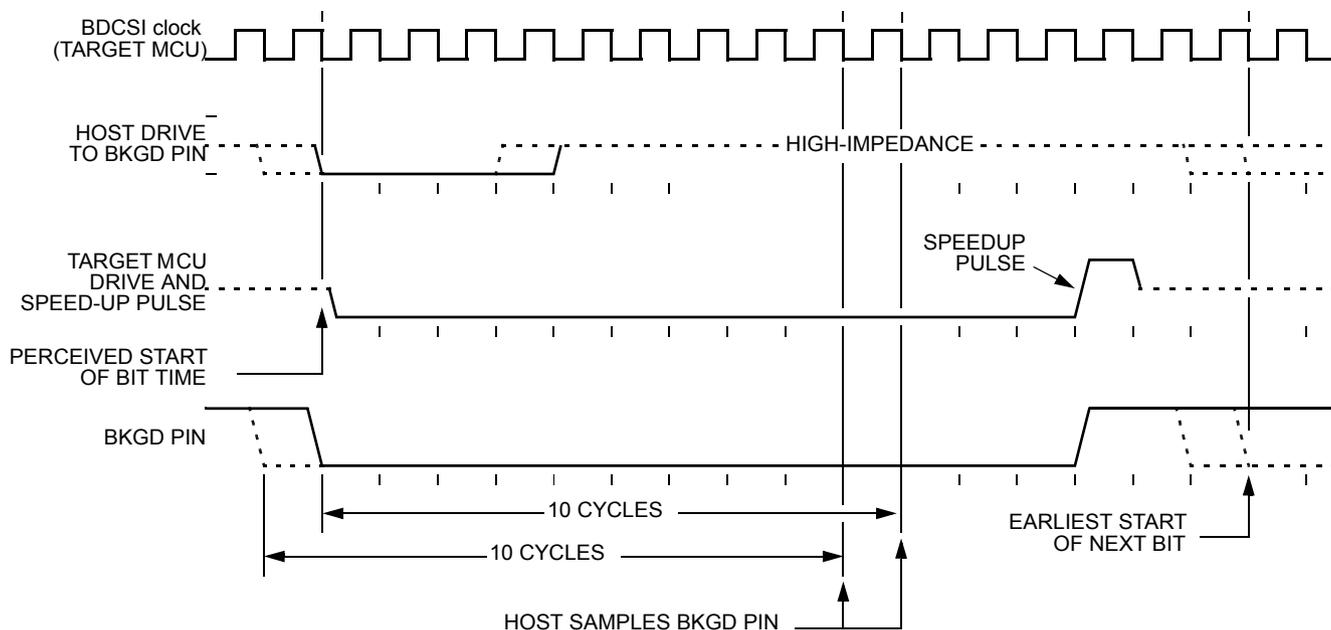
Figure 5-8. BDC Target-to-Host Serial Bit Timing (Logic 0)
