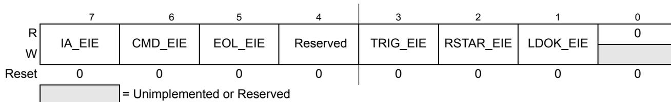
**Figure 10-10. ADC Error Interrupt Enable Register (ADCEIE)**
