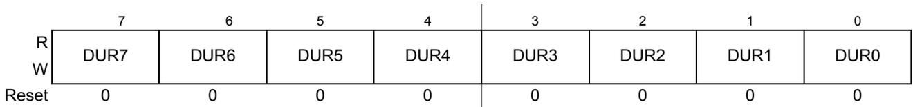
**Figure 19-15. SSG Tone Duration Register (SSGDUR)**
