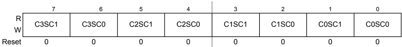
**Figure 6-10. Debug State Control Register 2 (DBGSCR2)**
