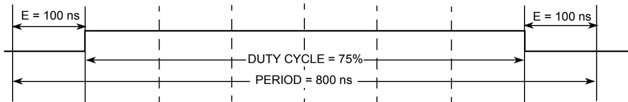
Figure 9-20. PWM Center Aligned Output Example Waveform
