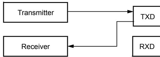
**Figure 15-30. Single-Wire Operation (LOOPS = 1, RSRC = 1)**
