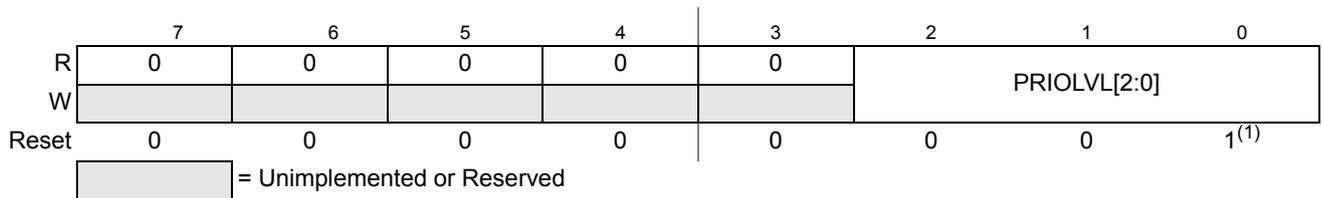
**Figure 4-10. Interrupt Request Configuration Data Register 5 (INT\_CFDATA5)**
