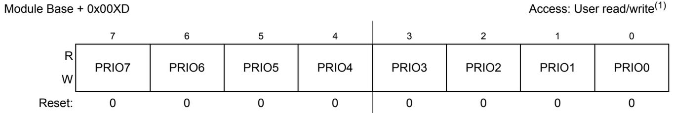
**Figure 11-36. Transmit Buffer Priority Register (TBPR)**
