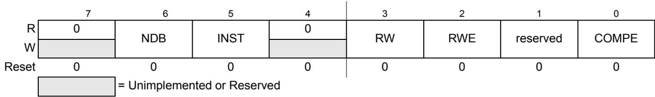
**Figure 6-20. Debug Comparator C Control Register**
