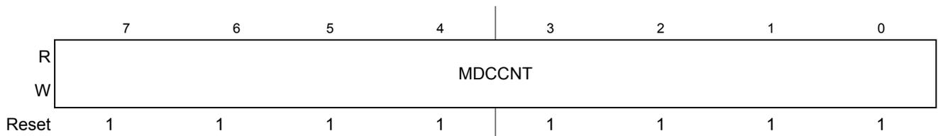
**Figure 17-7. Modulus Down-Counter Count Register Low (MDCCNT)**
