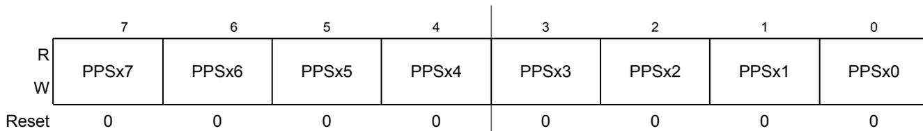
**Figure 2-11. Port S Polarity Select Register**
