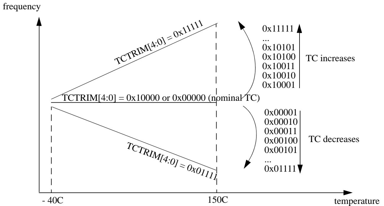
Figure 7-30. Influence of TCTRIM[4:0] on the Temperature Coefficient
