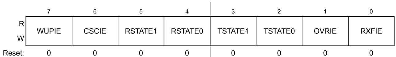
**Figure 11-9. MSCAN Receiver Interrupt Enable Register (CANRIER)**
