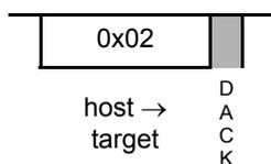
Enables the hardware handshake protocol in the serial communication. The hardware handshake is implemented by an acknowledge (ACK) pulse issued by the target MCU in response to a host command. The ACK\_ENABLE command is interpreted and executed in the BDC logic without the need to interface
