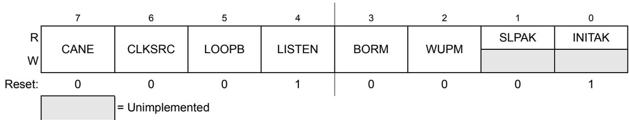
**Figure 11-5. MSCAN Control Register 1 (CANCTL1)**
