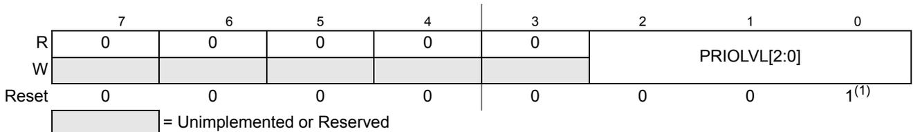
**Figure 4-7. Interrupt Request Configuration Data Register 2 (INT\_CFDATA2)**
