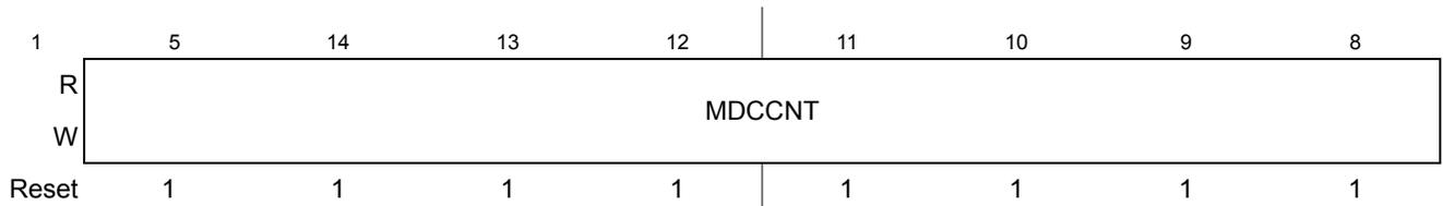
**Figure 17-6. Modulus Down-Counter Count Register High (MDCCNT)**
