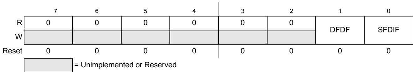
Figure 21-12. Flash Error Status Register (FERSTAT)
