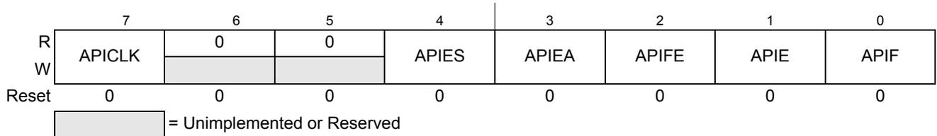
Figure 7-20. Autonomous Periodical Interrupt Control Register (CPMUAPICTL)
