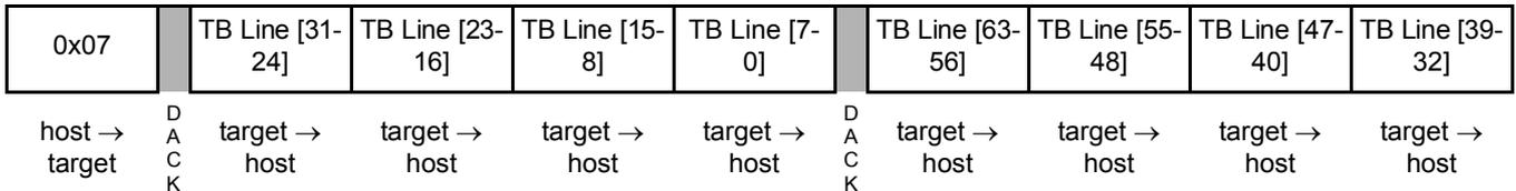
This command is only available on devices, where the DBG module includes a trace buffer. Attempted use of this command on devices without a trace buffer return 0x00.
