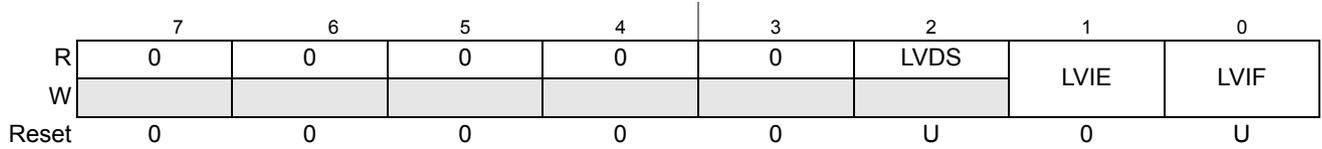
The Reset state of LVDS and LVIF depends on the external supplied VDDA level
