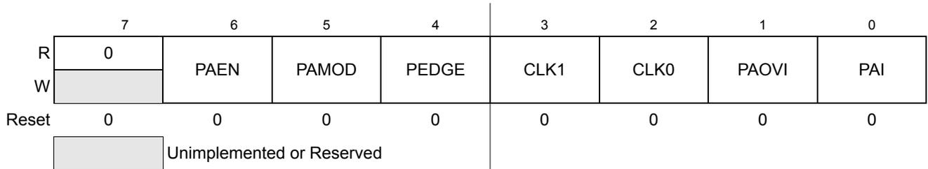
Figure 8-24. 16-Bit Pulse Accumulator Control Register (PACTL)
