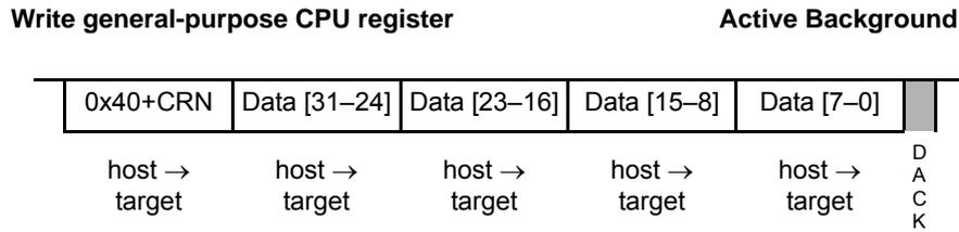
If the device is in active BDM, this command writes the 32-bit operand to the selected CPU general-purpose register. See [Section 5.4.5.1](#) for the CRN details. Accesses to CPU registers are always 32-bits wide, regardless of implemented register width. If enabled an ACK pulse is generated after the internal write access has been completed or aborted.
