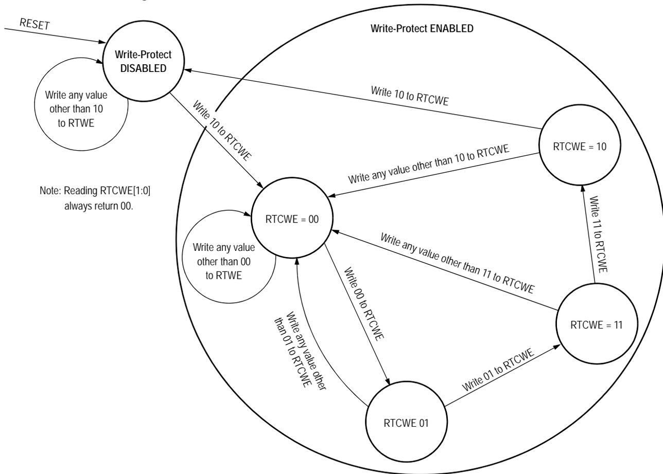
After a reset, the write-protect mechanism is disabled, allowing the user set the time and date in the calendar registers.
