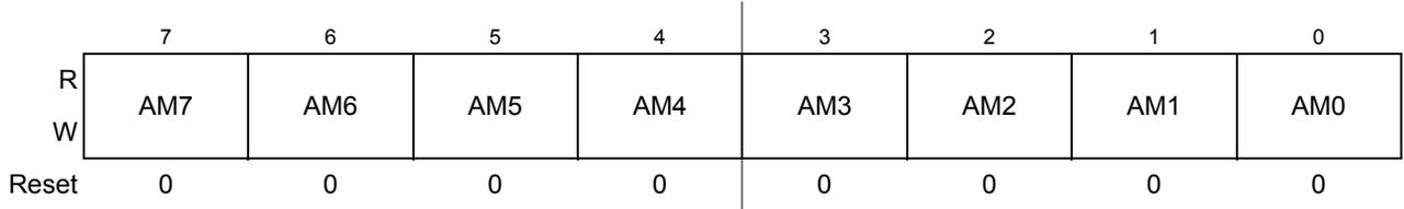
**Figure 11-22. MSCAN Identifier Mask Registers (First Bank) — CANIDMR0–CANIDMR3**
