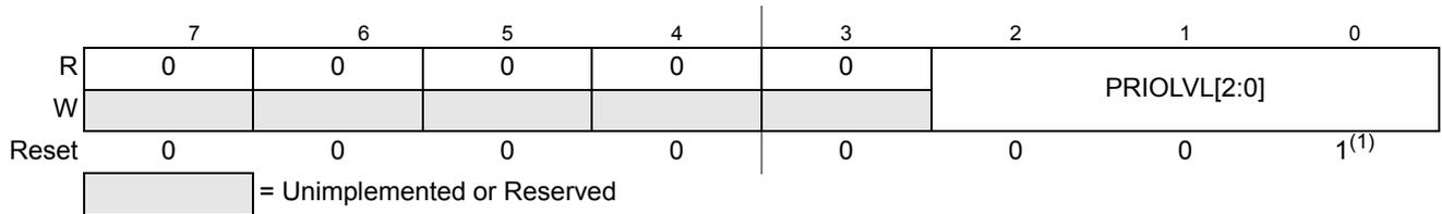
**Figure 4-8. Interrupt Request Configuration Data Register 3 (INT\_CFDATA3)**
