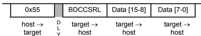
Read from location defined by the previous READ\_MEM. The previous READ\_MEM command defines the address, subsequent READ\_SAME commands return contents of same address. The example shows the sequence for reading a 16-bit word size. Byte alignment details are described in [Section 5.4.5.2](#). If enabled, an ACK pulse is driven before the data bytes are transmitted.
