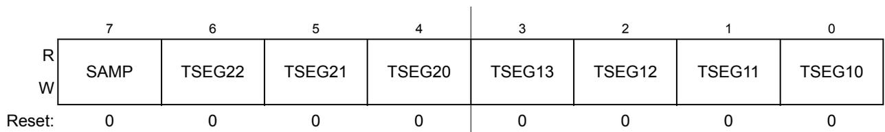
**Figure 11-7. MSCAN Bus Timing Register 1 (CANBTR1)**
