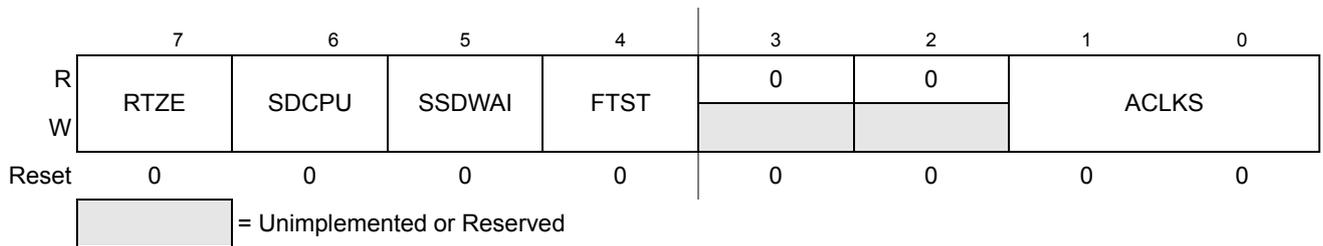
**Figure 17-4. Stepper Stall Detector Control Register (SSDCTL)**
