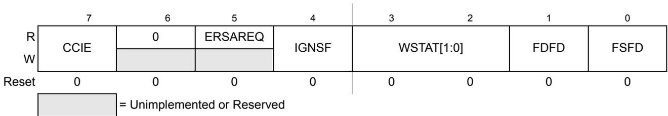
**Figure 21-9. Flash Configuration Register (FCNFG)**
