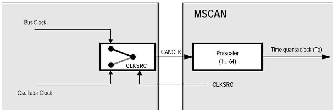
Figure 11-43. MSCAN Clocking Scheme
