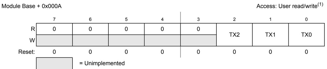
**Figure 11-14. MSCAN Transmit Buffer Selection Register (CANTBSEL)**
