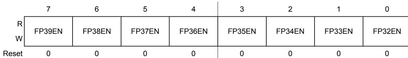
Figure 14-9. LCD Frontplane Enable Register 4 (LCDFPENR4)
