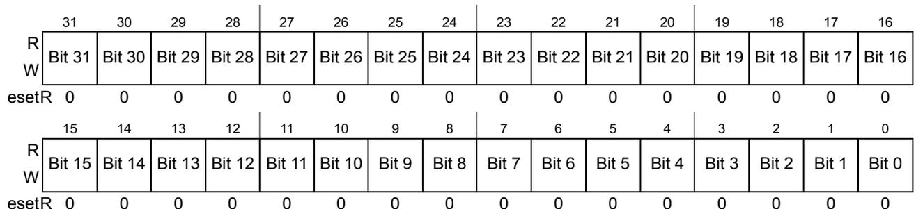
Figure 6-23. Debug Comparator C Data Mask Register (DBGCDM)
