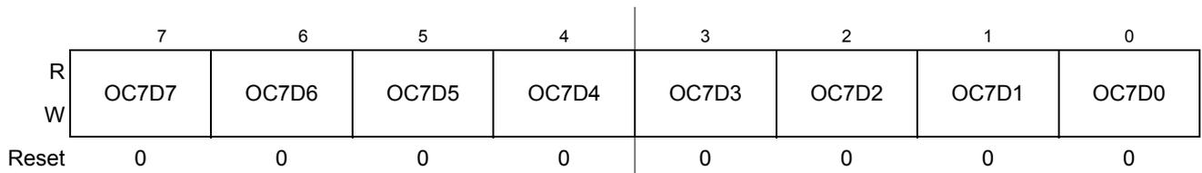
**Figure 8-9. Output Compare 7 Data Register (OC7D)**
