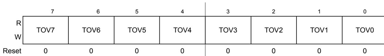
**Figure 8-13. Timer Toggle On Overflow Register 1 (TTOV)**
