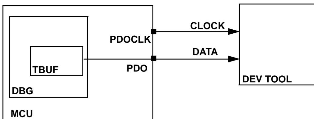
Figure 6-31 shows the profiling clock, PDOCLK, whose edges are offset from the bus clock, to ease setup and hold time requirements relative to PDO, which is synchronous to the bus clock.
