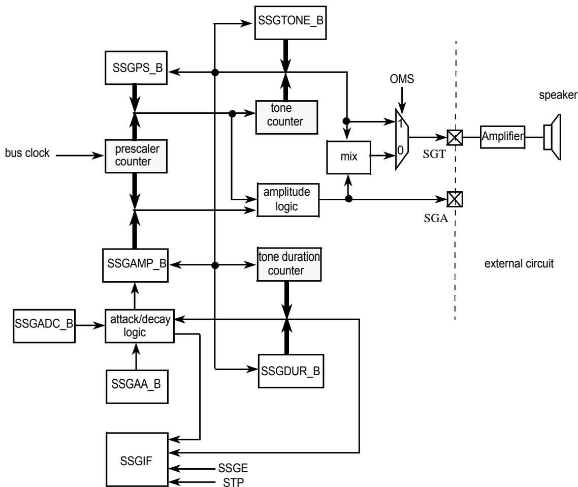
NOTE: XXX\_B is the buffer register of relevant XXX register
