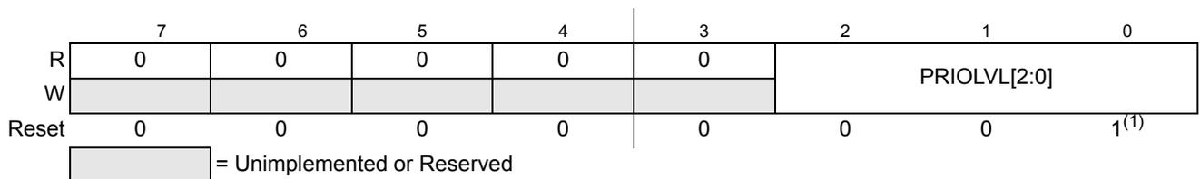
**Figure 4-11. Interrupt Request Configuration Data Register 6 (INT\_CFDATA6)**
