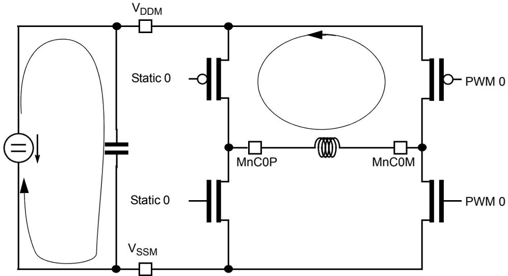
Figure 16-13. PWM Passive Phase, RECIRC = 0, S = 0
