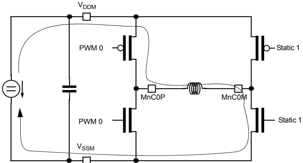
Figure 16-14. PWM Active Phase, RECIRC = 1, S = 0
