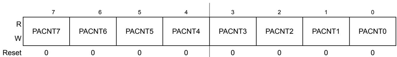
**Figure 8-27. Pulse Accumulator Count Register Low (PACNTL)**
