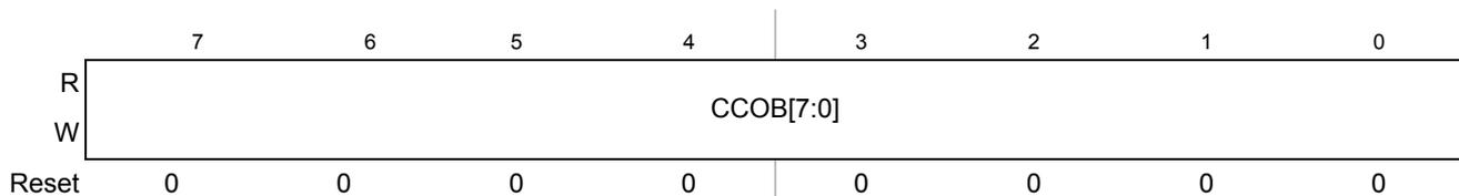
**Figure 21-21. Flash Common Command Object 1 Low Register (FCCOB1LO)**
