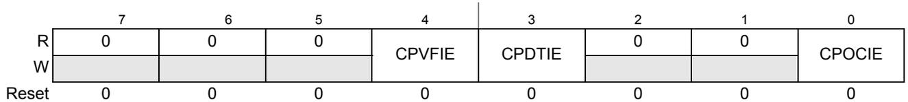
Figure 22-8. CAN Physical Layer Interrupt Enable Register (CPIE)
