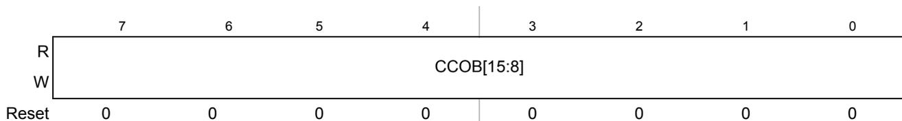
**Figure 21-24. Flash Common Command Object 3 High Register (FCCOB3HI)**
