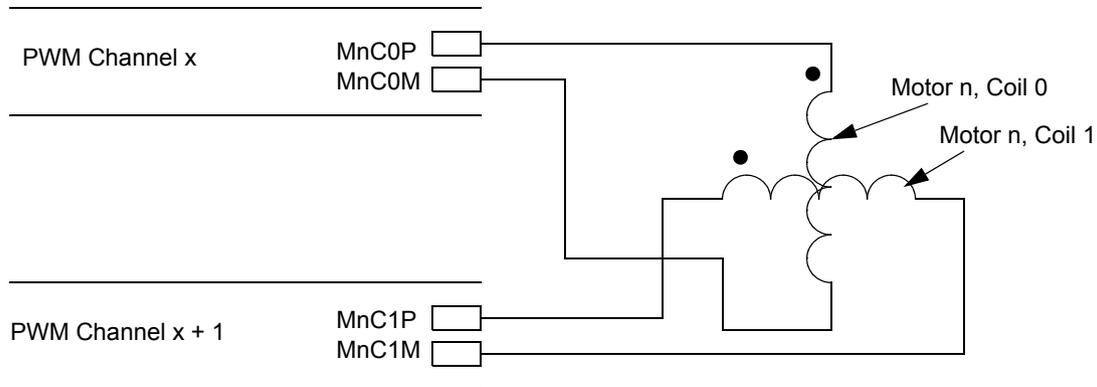
**Figure 16-10. Typical Dual Full H-Bridge Mode Configuration**
