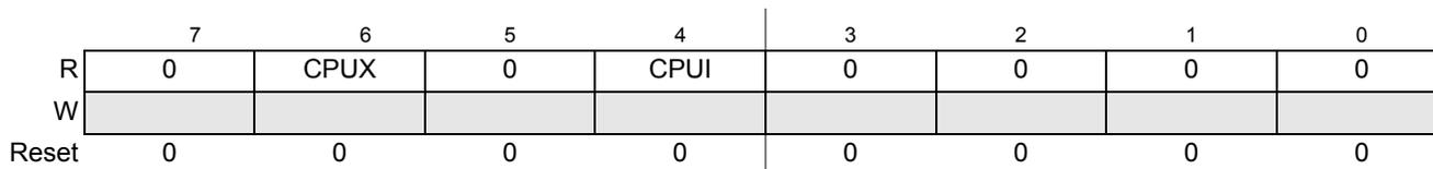
Figure 3-6. Captured S12ZCPU Condition Code Register (MMCCCRH, MMCCRL)
