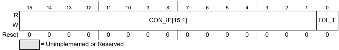
**Figure 10-14. ADC Conversion Interrupt Enable Register (ADCCONIE)**
