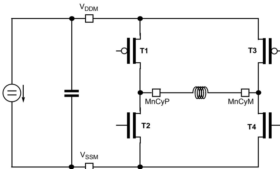
Figure 16-16. Output Transistor Assignment
