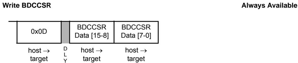
16-bit write to the BDCCSR register. No ACK pulse is generated. Writing to this register can be used to configure control bits or clear flag bits. Refer to the register bit descriptions.
