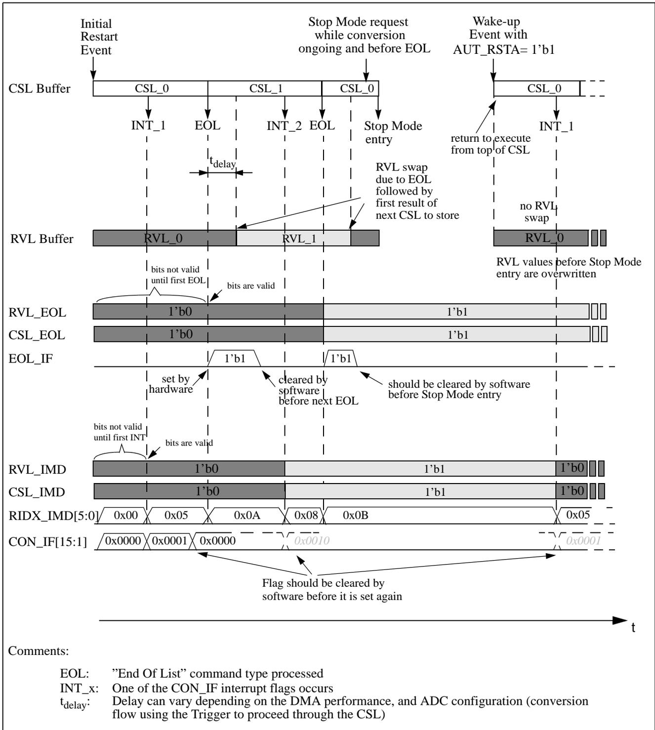
Figure 10-40. RVL Swapping — Use Case Diagram
