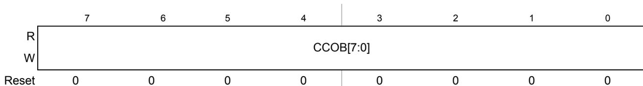
**Figure 21-27. Flash Common Command Object 4 Low Register (FCCOB4LO)**
