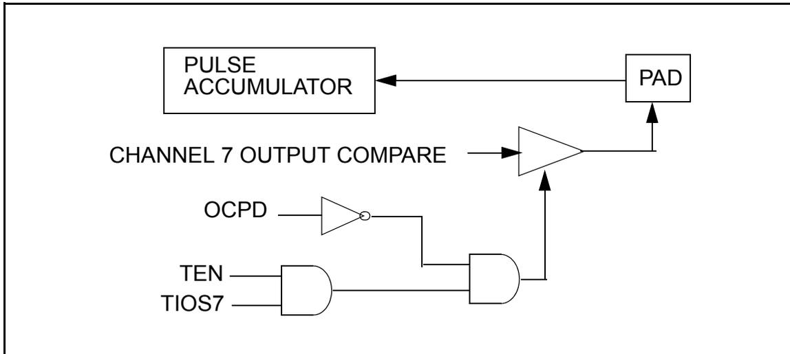
Figure 8-4. Channel 7 Output Compare/Pulse Accumulator Logic
