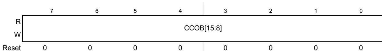
**Figure 21-20. Flash Common Command Object 1 High Register (FCCOB1HI)**
