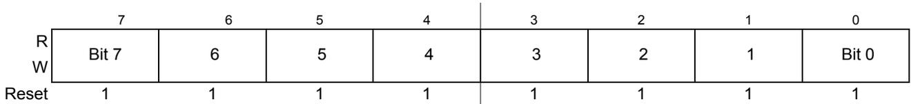
**Figure 9-14. PWM Channel Duty Registers (PWMDTY<sub>x</sub>)**
