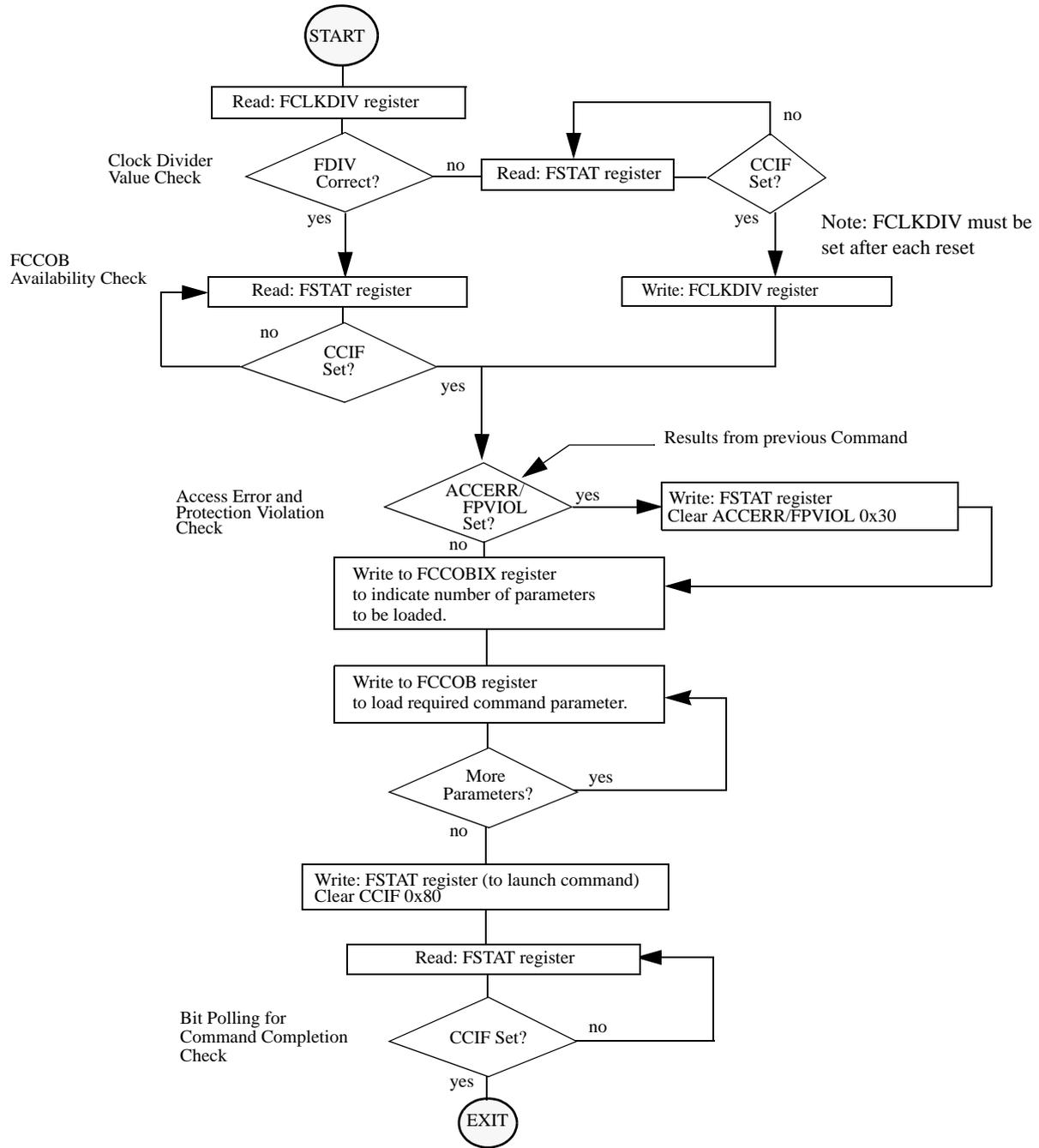
Figure 21-30. Generic Flash Command Write Sequence Flowchart
