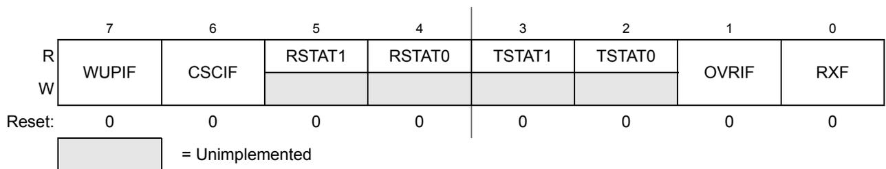
**Figure 11-8. MSCAN Receiver Flag Register (CANRFLG)**
