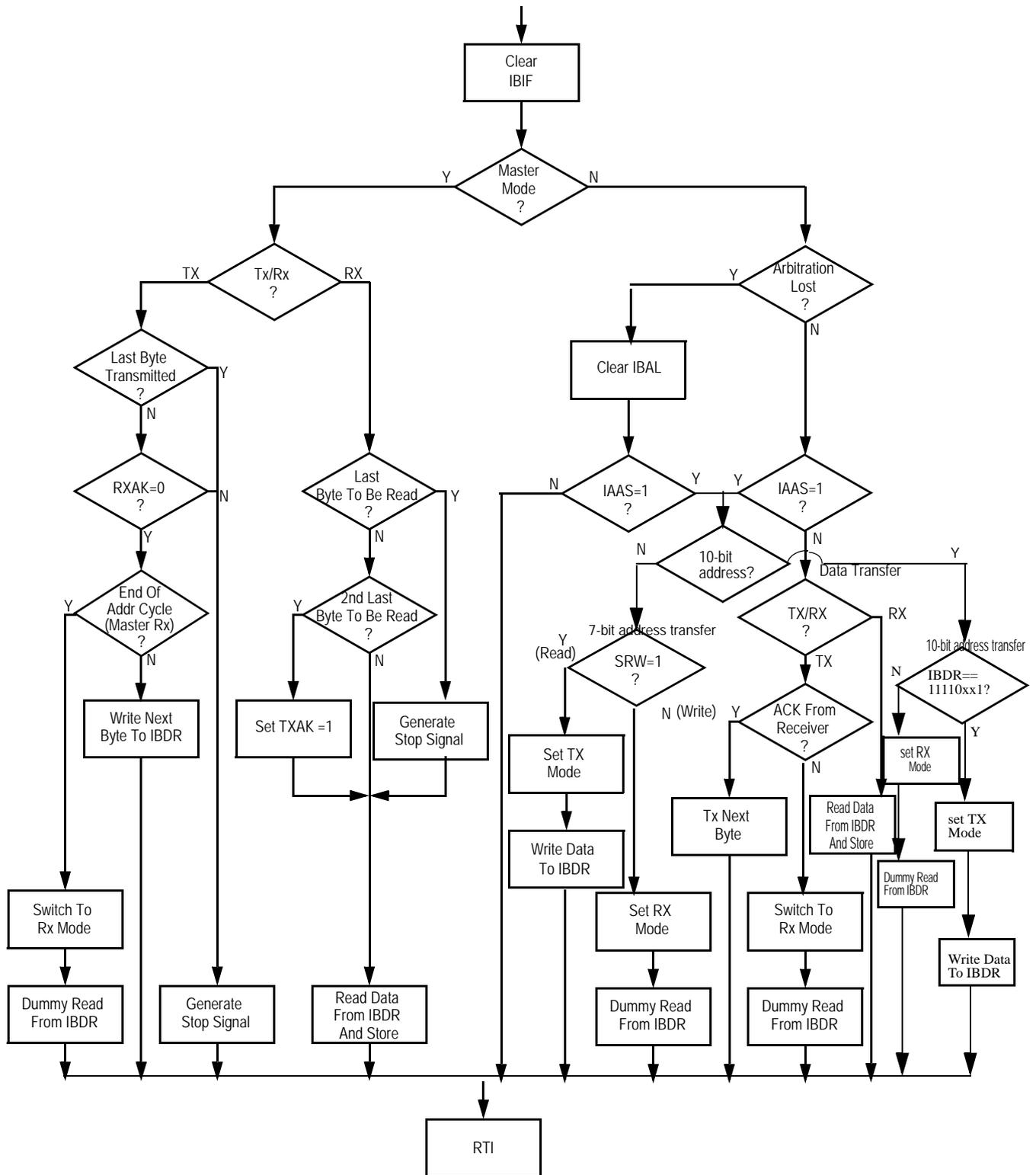
Figure 13-16. Flow-Chart of Typical IIC Interrupt Routine
