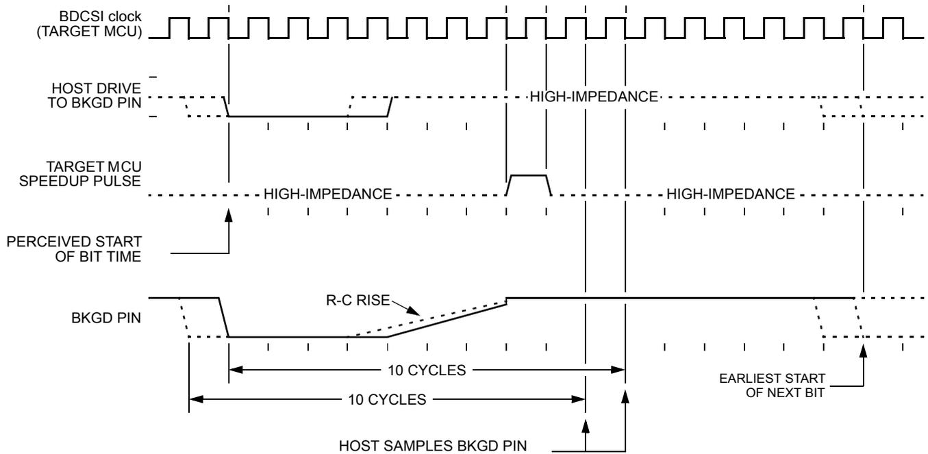
**Figure 5-7. BDC Target-to-Host Serial Bit Timing (Logic 1)**
