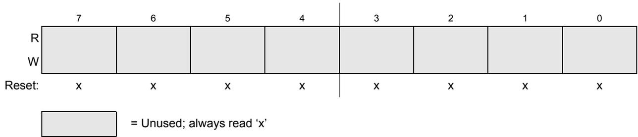
Figure 11-32. Identifier Register 2 — Standard Mapping
