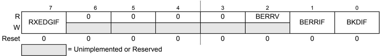
**Figure 15-6. SCI Alternative Status Register 1 (SCIASR1)**
