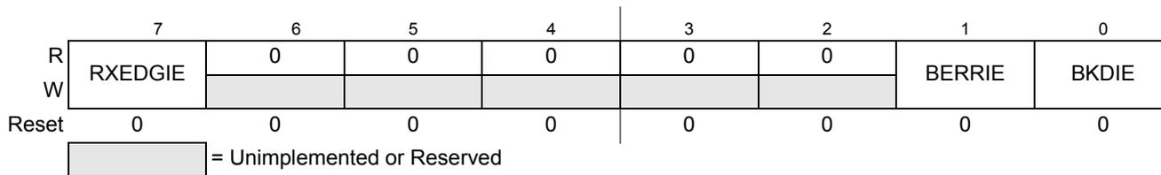
**Figure 15-7. SCI Alternative Control Register 1 (SCIACR1)**
