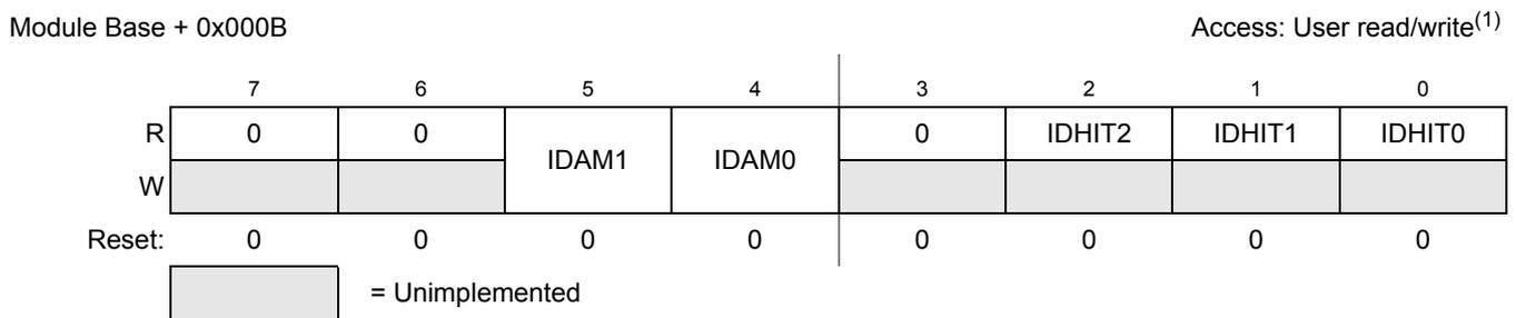
**Figure 11-15. MSCAN Identifier Acceptance Control Register (CANIDAC)**
