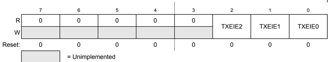
**Figure 11-11. MSCAN Transmitter Interrupt Enable Register (CANTIER)**
