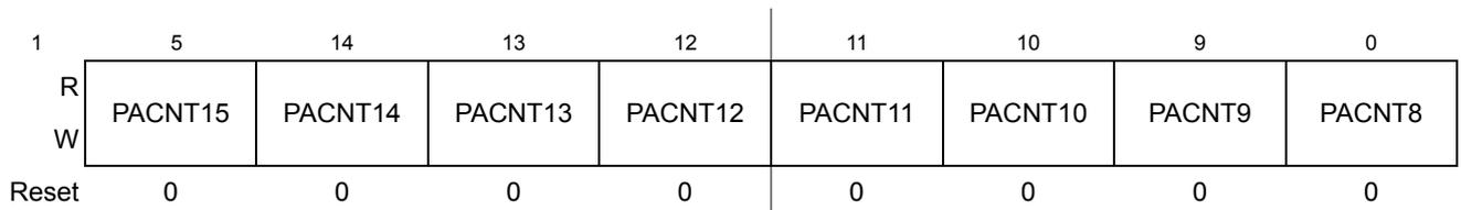
**Figure 8-26. Pulse Accumulator Count Register High (PACNTH)**
