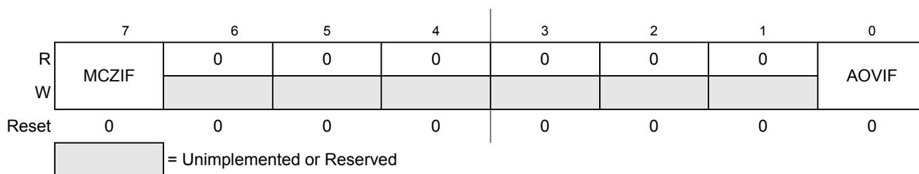
**Figure 17-5. Stepper Stall Detector Flag Register (SSDFLG)**
