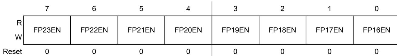
Figure 14-7. LCD Frontplane Enable Register 2 (LCDFPENR2)
