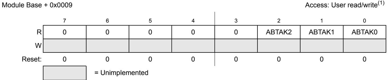
**Figure 11-13. MSCAN Transmitter Message Abort Acknowledge Register (CANTAACK)**
