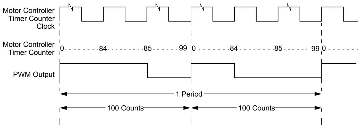
**Figure 16-20. PWM Output: DITH = 1, MCAM[1:0] = 10, MCDC = 31, MCPER = 200, RECIRC = 0**
