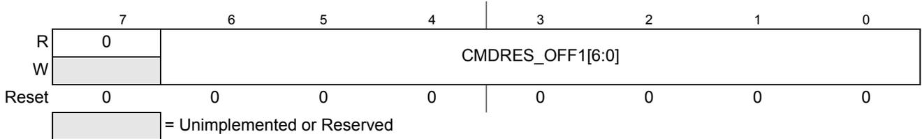
**Figure 10-27. ADC Command and Result Offset Register 1 (ADCCROFF1)**
