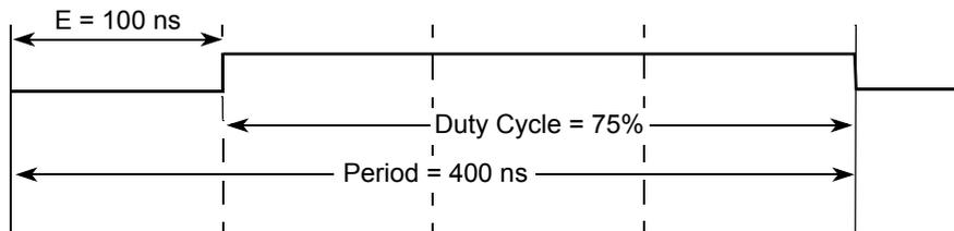
Figure 9-18. PWM Left Aligned Output Example Waveform
