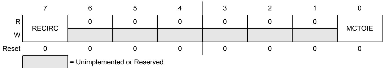
**Figure 16-4. Motor Controller Control Register 1 (MCCTL1)**
