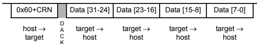
This command reads the selected CPU registers and returns the 32-bit result. Accesses to CPU registers are always 32-bits wide, regardless of implemented register width. Bytes that are not implemented return
