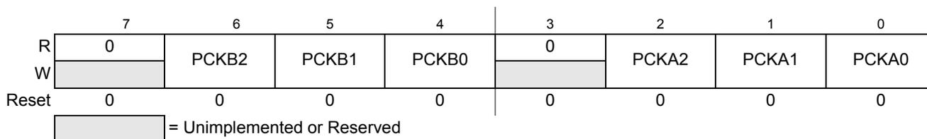
**Figure 9-6. PWM Prescale Clock Select Register (PWMPRCLK)**
