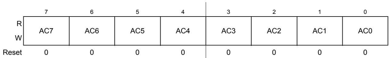
**Figure 11-20. MSCAN Identifier Acceptance Registers (First Bank) — CANIDAR0–CANIDAR3**
