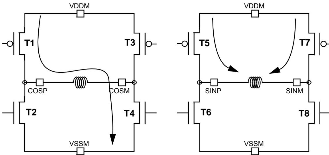
Figure 17-11. Current Flow when STEP = 0, DCOIL = 1, ITG = 0, RCIR = 0
