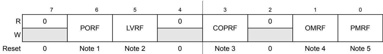
1. PORF is set to 1 when a power on reset occurs. Unaffected by System Reset.
