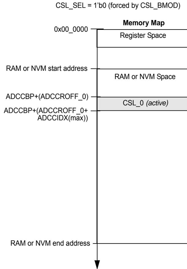
**Note:** Address register names in () are not absolute addresses instead they are a sample offset or sample index
