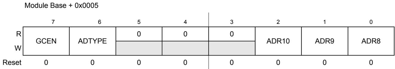
Figure 13-9. IIC Bus Control Register 2(BCR2)
