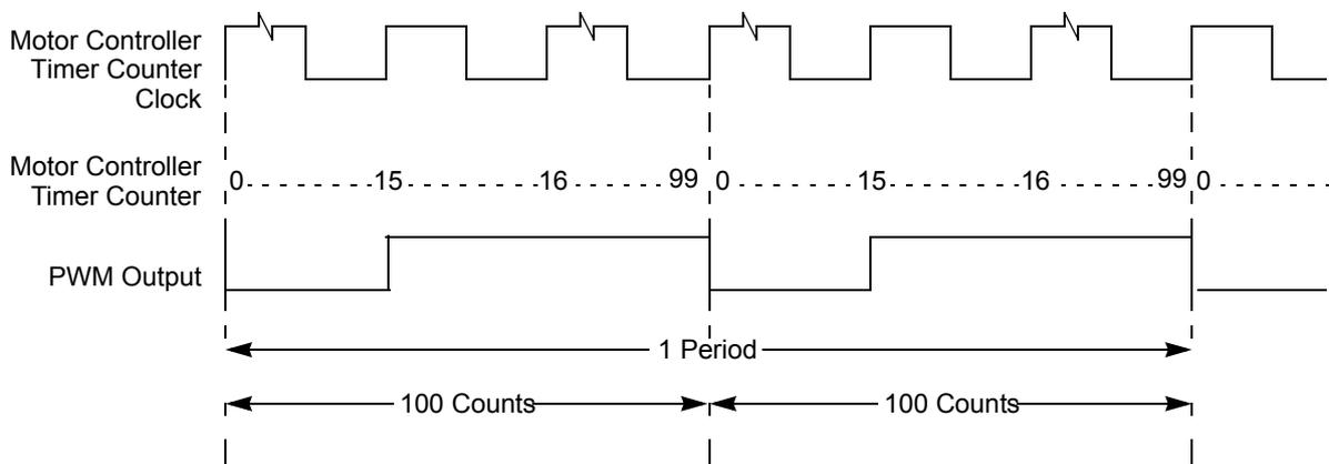
**Figure 16-19. PWM Output: DITH = 1, MCAM[1:0] = 01, MCDC = 30, MCPER = 200, RECIRC = 0**
