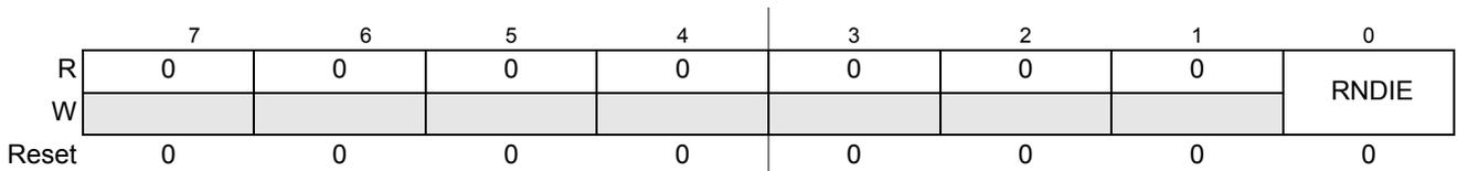
**Figure 19-16. SSG Interrupt Enable Register (SSGIE)**
