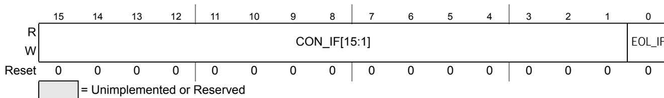
Figure 10-15. ADC Conversion Interrupt Flag Register (ADCCONIF)
