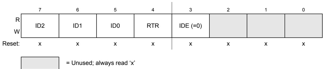
**Figure 11-31. Identifier Register 1 — Standard Mapping**
