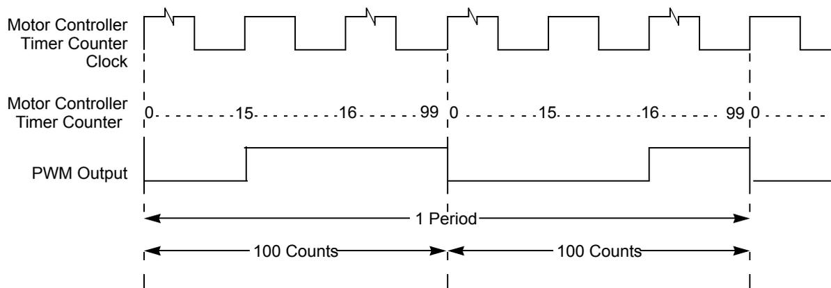
Figure 16-18. PWM Output: DITH = 1, MCAM[1:0] = 01, MCDC = 31, MCPER = 200, RECIRC = 0
