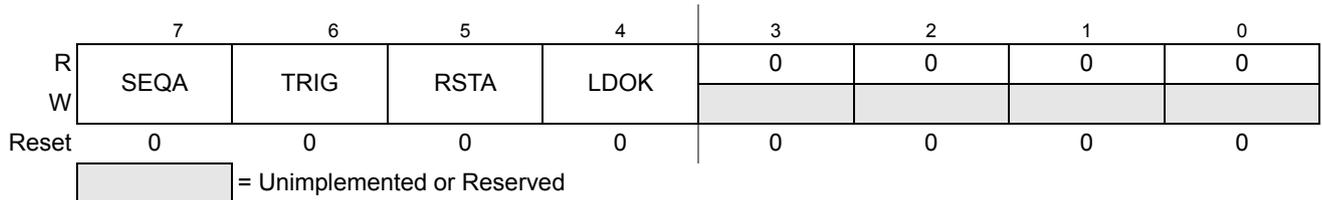
**Figure 10-9. ADC Conversion Flow Control Register (ADCFLWCTL)**
