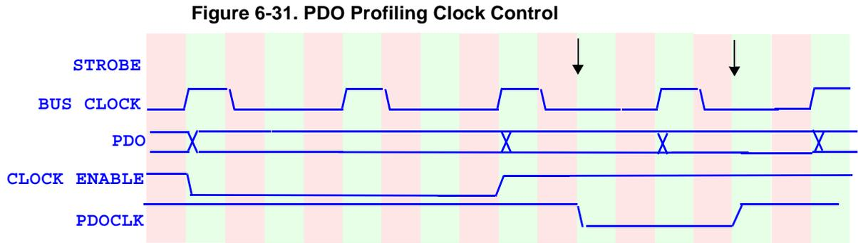
The trace buffer is used as a temporary storage medium to store COF information before it is transmitted. COF information can be transmitted whilst new information is written to the trace buffer. The trace buffer data is transmitted at PDO least significant bit first. After the first trace buffer entry is made, transmission begins in the first clock period in which no further data is written to the trace buffer.
