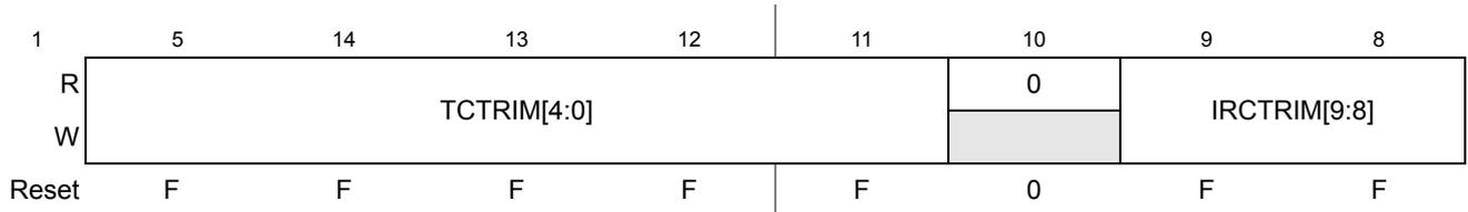
After de-assert of System Reset a factory programmed trim value is automatically loaded from the Flash memory to provide trimmed Internal Reference Frequency  $f_{IRC1M\_TRIM}$ .
