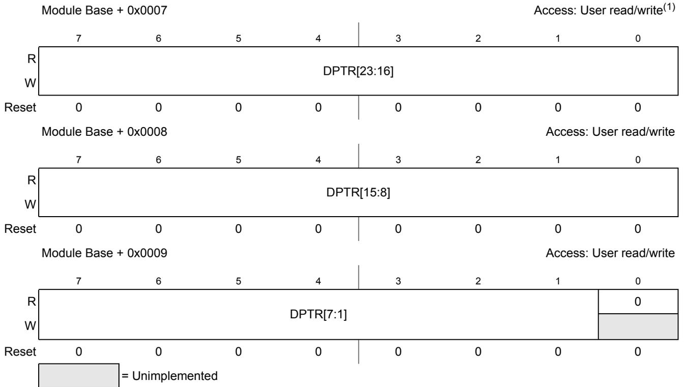
**Figure 20-5. ECC Debug Pointer Register (ECCDPTRH, ECCDPTRM, ECCDPTRL)**
