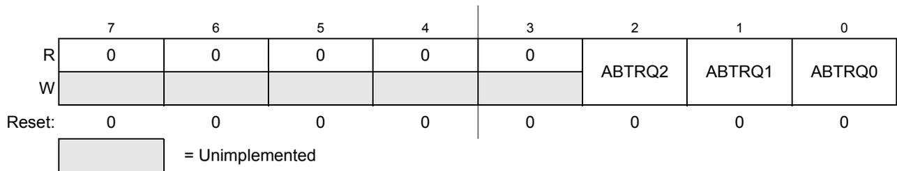
**Figure 11-12. MSCAN Transmitter Message Abort Request Register (CANTARQ)**
