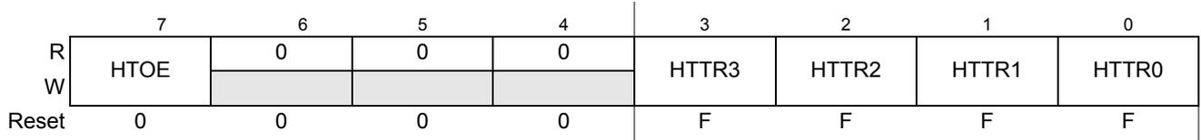
After de-assert of System Reset a trim value is automatically loaded from the Flash memory. See Device specification for details.
