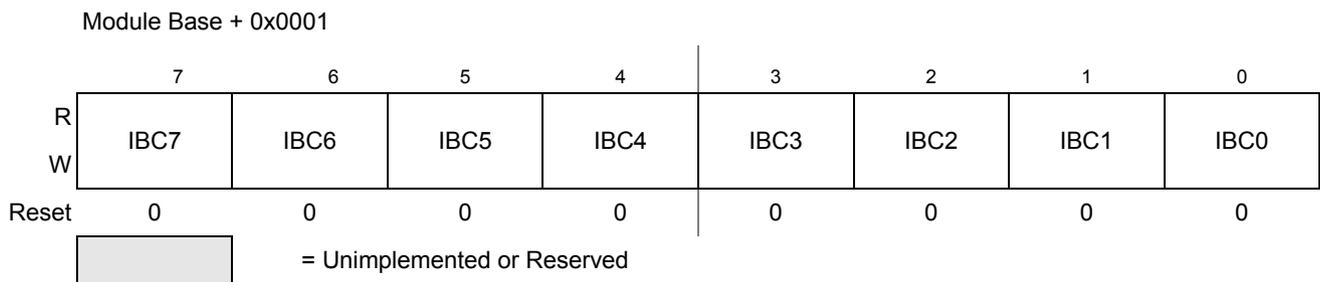
**Figure 13-4. IIC Bus Frequency Divider Register (IBFD)**
