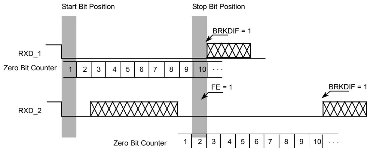
Figure 15-17. Break Detection if BRKDFE = 1 (M = 0)
