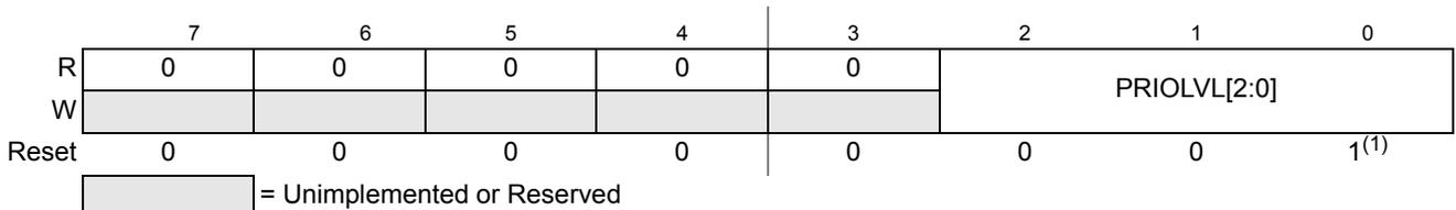
**Figure 4-6. Interrupt Request Configuration Data Register 1 (INT\_CFDATA1)**
