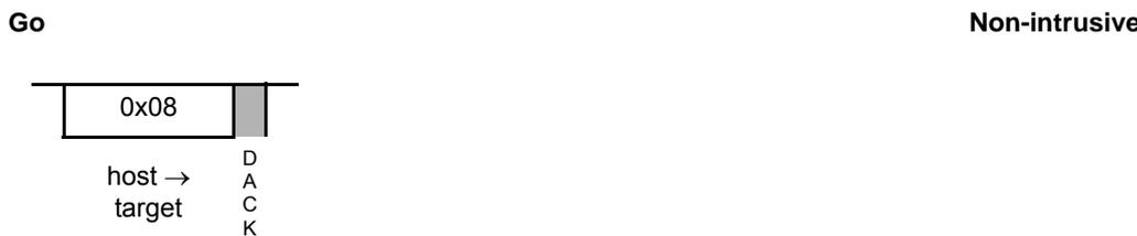
This command is used to exit active BDM and begin (or resume) execution of CPU application code. The CPU pipeline is flushed and refilled before normal instruction execution resumes. Prefetching begins at the current address in the PC. If any register (such as the PC) is altered by a BDC command whilst in BDM, the updated value is used when prefetching resumes. If enabled, an ACK is driven on exiting active BDM.
