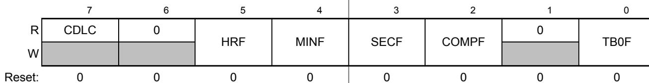
**Figure 18-6. RTC Status and Control Register1 (RTCS1)**
