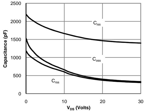
**Figure 8: Capacitance Characteristics**
