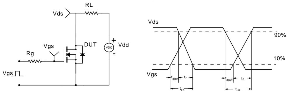
**Unclamped Inductive Switching (UIS) Test Circuit & Waveforms**
