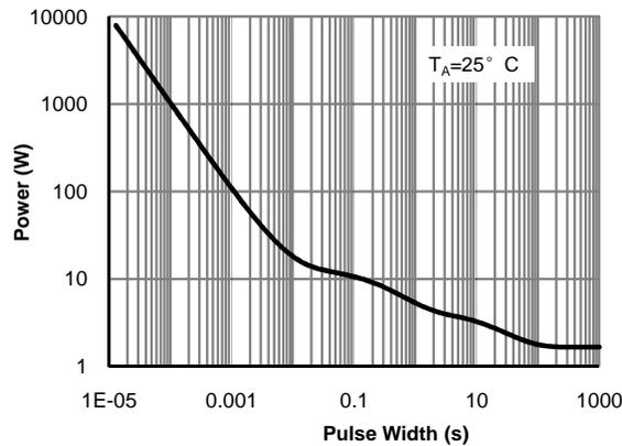
Figure 14: Single Pulse Power Rating Junction-to-Ambient (Note H)
