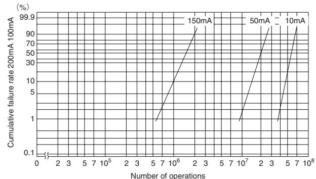
\* Arrow indicates number of operations where test was completed.
