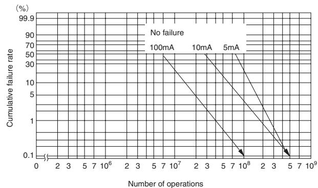
\* Arrow indicates number of operations where test was completed.
