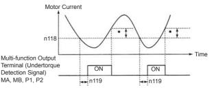
\* Undertorque detection release width (hysteresis) is set at approx. 5 % of the Inverter's rated current.
