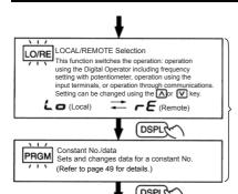
If the V7AZ is stopped after it has changed to any of these modes during operation, it changes to Program mode from Drive mode. Even if the Run Command is turned ON again, the V7AZ does not operate. However, if n001=5, the Run Command can be received and the V7AZ will operate.
