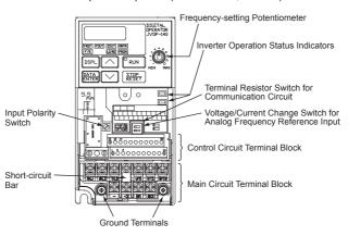
Example for 3-phase (200 V Class, 0.1 kW) Inverter
