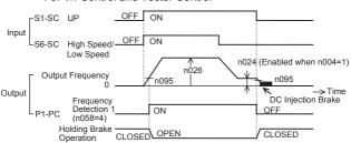
• For a variable speed operation by an analog signal, set the Frequency Reference Selection (n004) to a value from 2 to 4.
