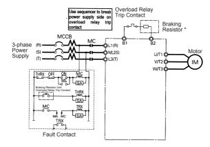
\* Disable stall prevention during deceleration by setting n092 to 1 when using a Braking Resistor Unit. The motor may not stop within the deceleration time if this setting is not changed.
