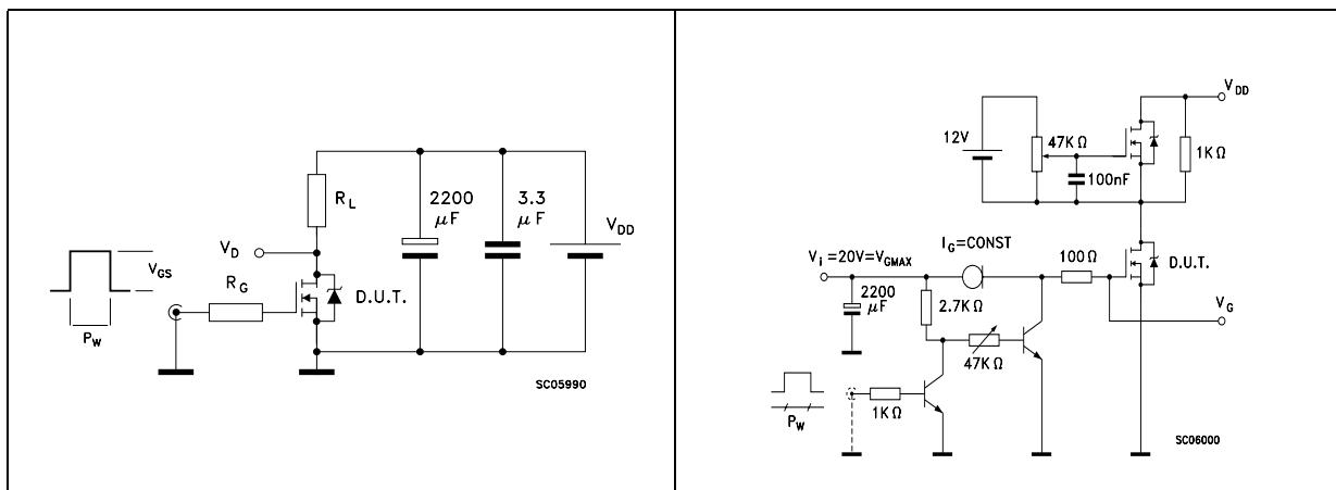
**Figure 19. Gate charge test circuit**
