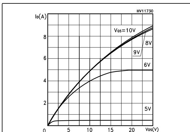
Figure 6. Transfer characteristics
