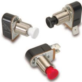
The P27-Series pushbutton switches are single pole, AC rated switches suitable for general purpose applications with a shallow back panel. These switches are momentary action with a medium actuation force (26 oz. typical). The P27-Series switch is equipped with a slow-make, slow-break contact mechanism, rated at 6 amps with a nylon concave pushbutton.
