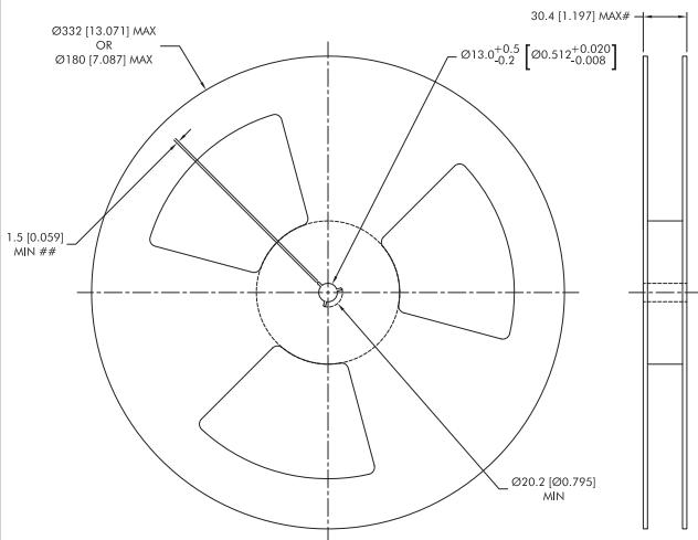
Tape & Reel specifications shall conform with current EIA-481 standard
