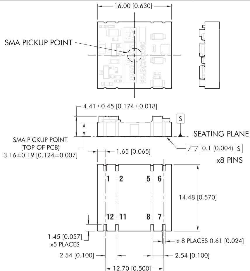
All dimensions in mm(inches), Controlling dimension is mm. Tolerances (unless otherwise stated)  $\pm 0.2$  (0.008).
