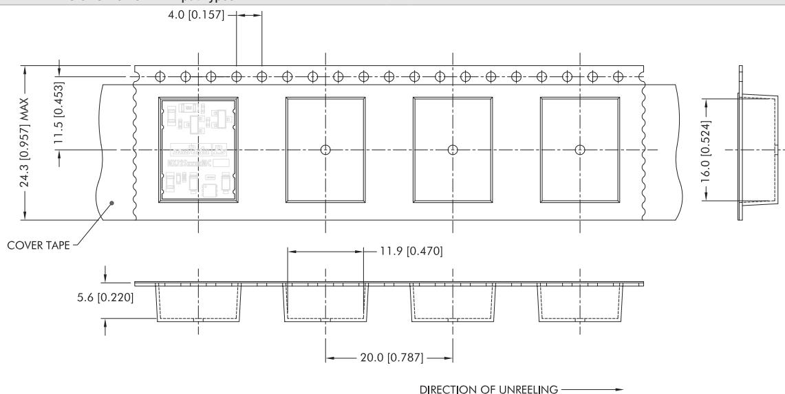
Tape & Reel specifications shall conform with current EIA-481 standard
