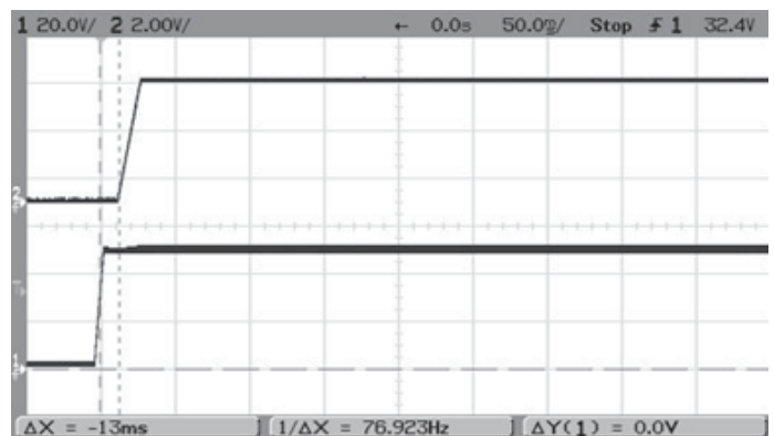
Start-up Delay (Vin = 48V, Vout = nom, Iout = 40A, Cload = 0, Ta = +25°C) ch1 = Vin, ch2 = Vout
