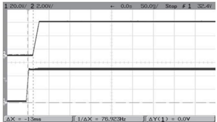
Start-up Delay (Vin = 48V, Vout = nom, Iout = 40A, Cload = 10000µf, Ta = +25°C) ch1 = Vin, ch2 = Vout
