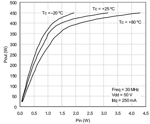
Figure 9: Power gain vs. output power
