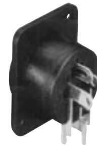
PD3FRA1 3-contact female, right-angle (bottom exit) PC/solder terminals. Ground lug. Front panel mount.
