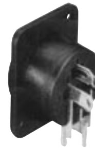
PD3FRA1 3-contact female, right-angle (bottom exit) PC/solder terminals. Ground lug. Front panel mount.
