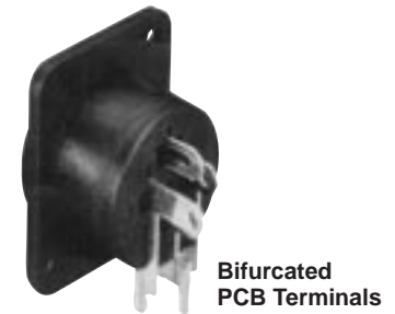
PD3FRA1 3-contact female, right-angle (bottom exit) PC/solder terminals. Ground lug. Front panel mount.
