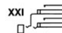
Double open circuit. Isolated switching—separate "make" circuits on both tip and ring. (J2-2A).
