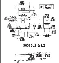
RECOMMENDED PC BOARD **LAYOUT (Component Side)**
