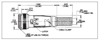
Non-reflective metal shell; 2 through 5 pins (male) or 2 through 5 contacts (female). Also 2-, 3- and 4-contact inserts with two shunted (N.C.) contacts. Efficient cable clamp and strain relief.
