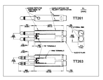
**TT263:** 6-circuit plug consists of two electrically-independent 3-conductor fingers with black handle. Can use single or dual cables for two electrically-independent 3-conductor fingers or common tip, ring and/or sleeve circuits.
