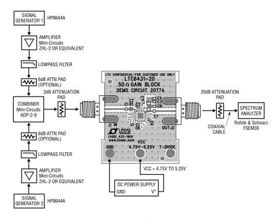
Figure 3. Proper Equipement Setup for IP3 Measurement
