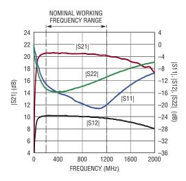
Figure 2. Demo Board S-Parameters
