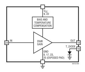
Figure 1. LTC6431-20 Device Block Diagram
