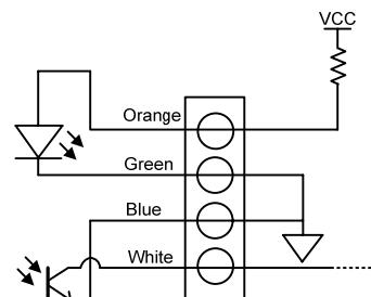
Figure 2 Sensor Connection Diagram
