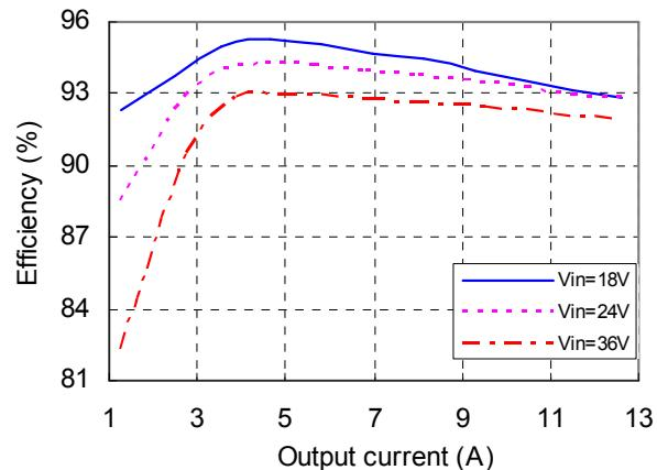
Figure 1 Efficiency vs. output current,  $T_a=25^\circ\text{C}$ ,  $T_c<40^\circ\text{C}$ ,  $V_o=28\text{V}$
