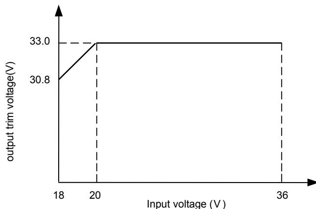
Figure 14 Output trim voltage vs. input voltage
