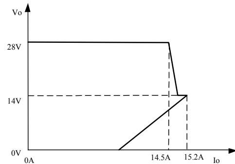
Figure 9 Over-current protection characteristics
