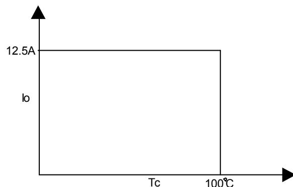
Figure 19 Output power derating, 24V<sub>in</sub>
